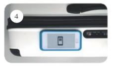
Align the BAGTAG directly above the desired area on your bag and press the device firmly onto the bag. Let the BAGTAG device cure for 24 hours.
