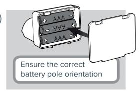
Fit 3x AAA batteries and replace the battery door, check the LED's status.
