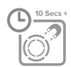
Hold the magnet over the device for 10 seconds, until the status LED turns red
