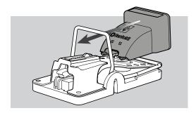
Slide Module back onto the base
