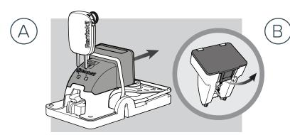
Ensure the trap is disarmed, then remove Main Assembly from shoe using RI Service Key and remove the battery door.
