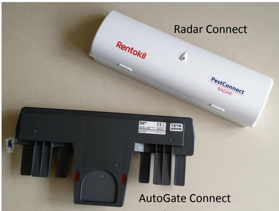
Figure 1: Connect System Overview
