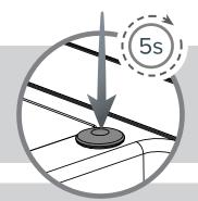
Press and hold button for five seconds to go into the 'A' Mode settings. Once in this mode press the button to cycle between detection options
