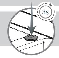
To move to LED Test, press and hold the button for three seconds. To exit the Diagnostic Mode, you must remove the battery and reinsert it.
