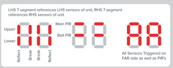
The Eradico Gate Connect device has "Near" IR sensors - those IR sensors which sit either side of the gate, and "FAR" Sensors - those IR sensors that sit opposite to the gate. When displaying the NEAR IR status, the bottom LED bar will be illuminated, when displaying the FAR IR status, the bottom LED bars will not be illuminated. To switch between the status of NEAR and FAR Sensors, press the button.
