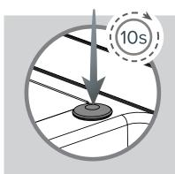
If you entered Diagnostic Mode from the Service and Maintenance section on Page 15, then skip this section. Otherwise go up to the device and press the button once. You will then either see an Error code or Device Status (Icon ♥). At which point press and hold the button for ten seconds and the display will count up, release when it gets to ten.
