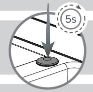
Press and hold button for five seconds to go into the 'B' Mode settings.
