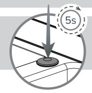
Press and hold button for five seconds to go into the 'C' Mode settings.
