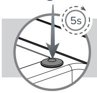
To enter Configuration Mode hold the button down for five seconds when in Service Mode, or after first inserting the battery pack.
