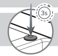
To go back to Sensor Test, press and hold the button for three seconds. To exit the Diagnostic Mode, you must remove the battery and reinsert it.
