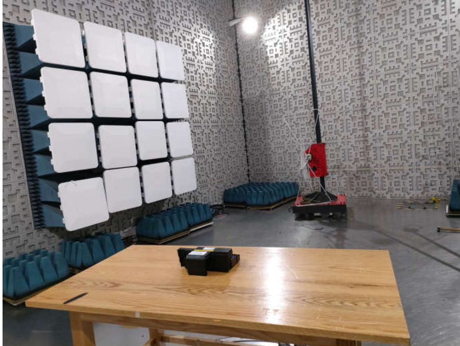
Radiated spurious emission Test Setup-1(Below 1GHz)
