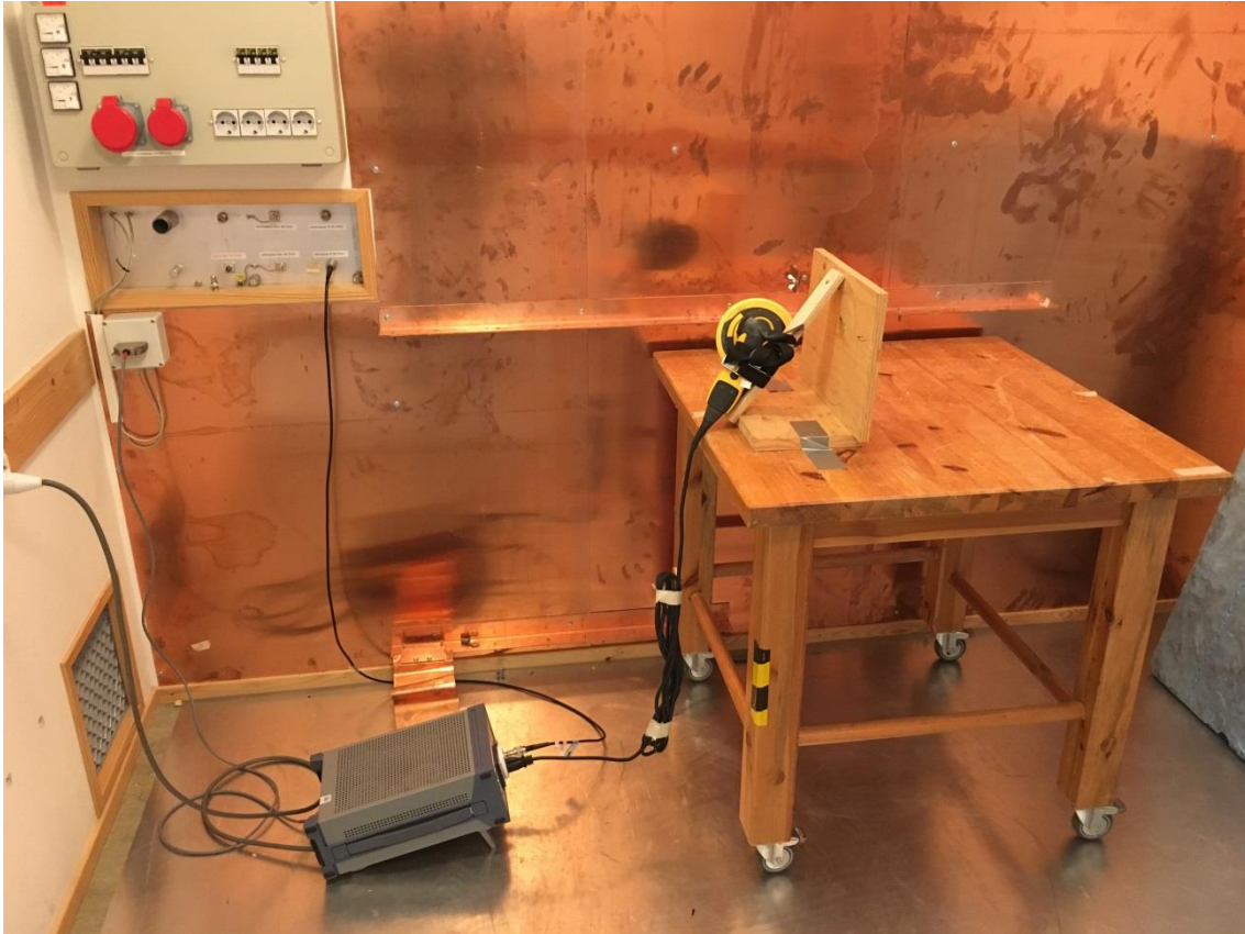
Test set up conducted emission 150 kHz – 30 MHz
