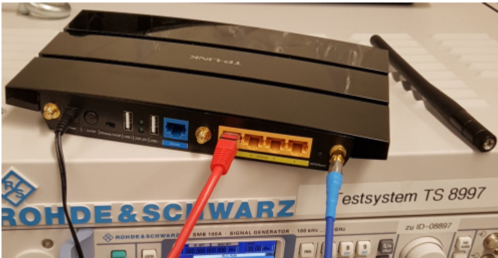
Figure 23: Connection of Router
