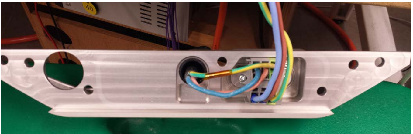
Figure 19: Connection of a cable to the cage clamp in the service flap
