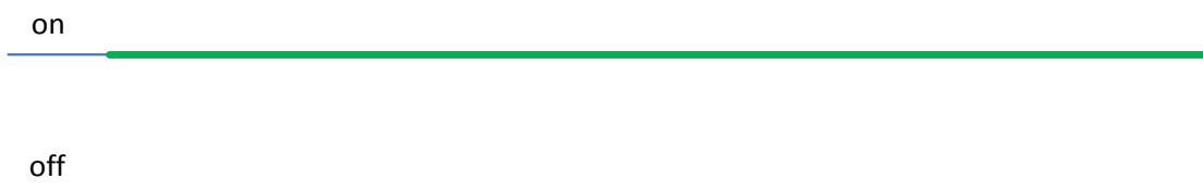
Figure 6: Flashing pattern in status Connected
