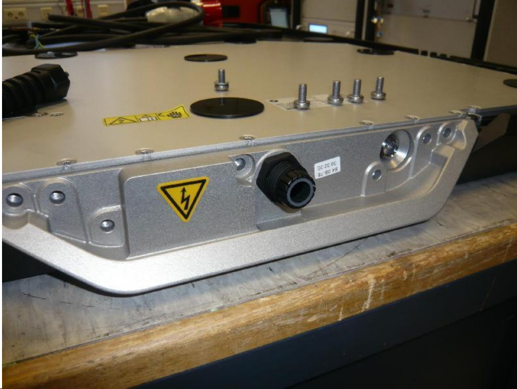
Bild / Picture 29: GPM – infeed main supply cable
