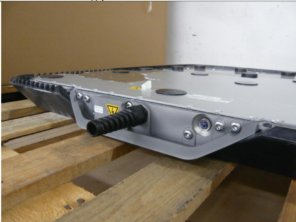
Bild / Picture 28: GPM – infeed main supply cable
