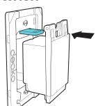
While pressing the switch inwards, push in the blue tab If the backplate is powered, the switch will flash ogreen If switch does not flash green, move to the next location & repeat step 1 15 Wait until the switch stops flashing green, then press & hold the configure button until it flashes • purple
