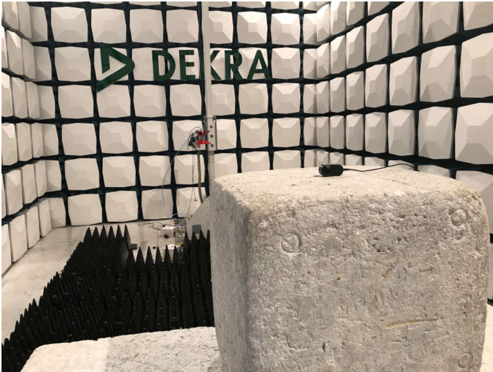
Description: Radiated Emission Test Setup for 1~18GHz
