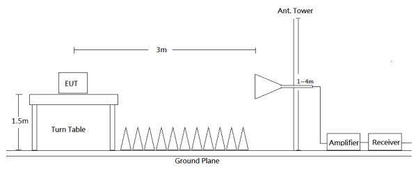
Radiated emission tests were performed in the 3 meters chamber test site, using the setup accordance with the ANSI C63.10-2013. The specification used was the FCC 15.205, FCC 15.209, FCC 15.249 and RSS-GEN, RSS-210 limits.
