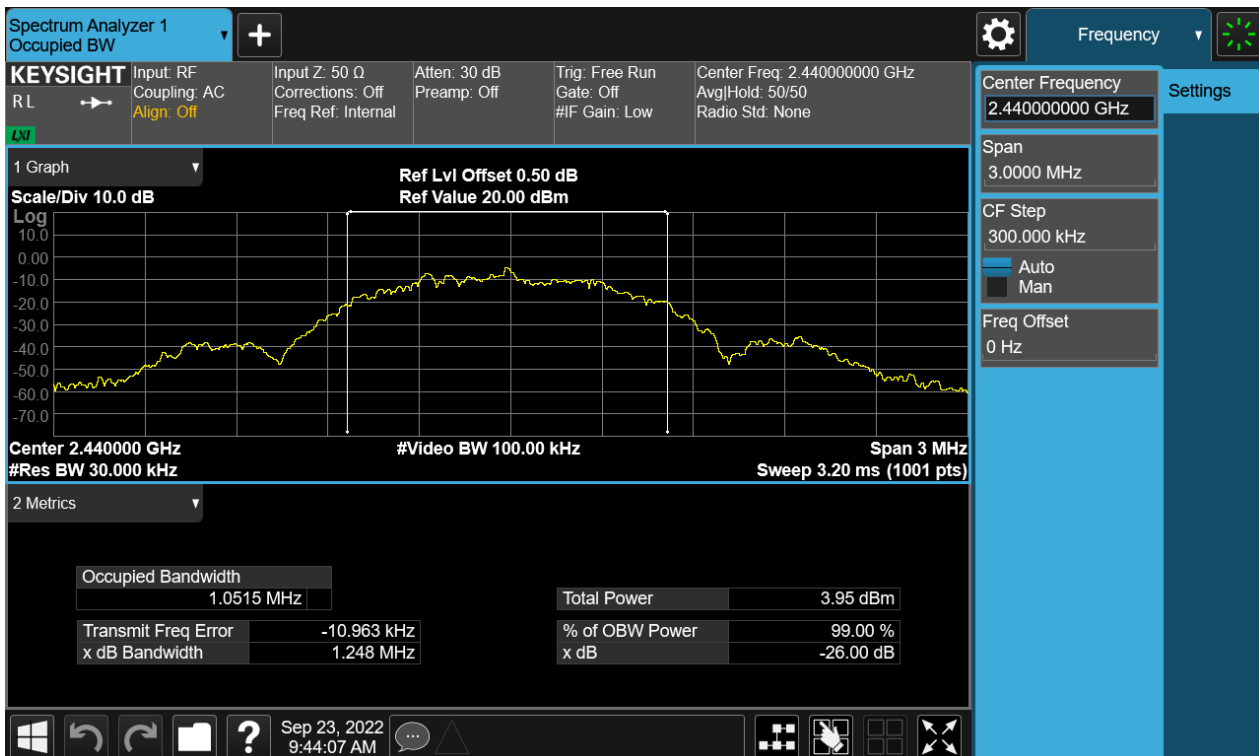
Figure 7: The plots of 99% Bandwidth, 2440MHz
