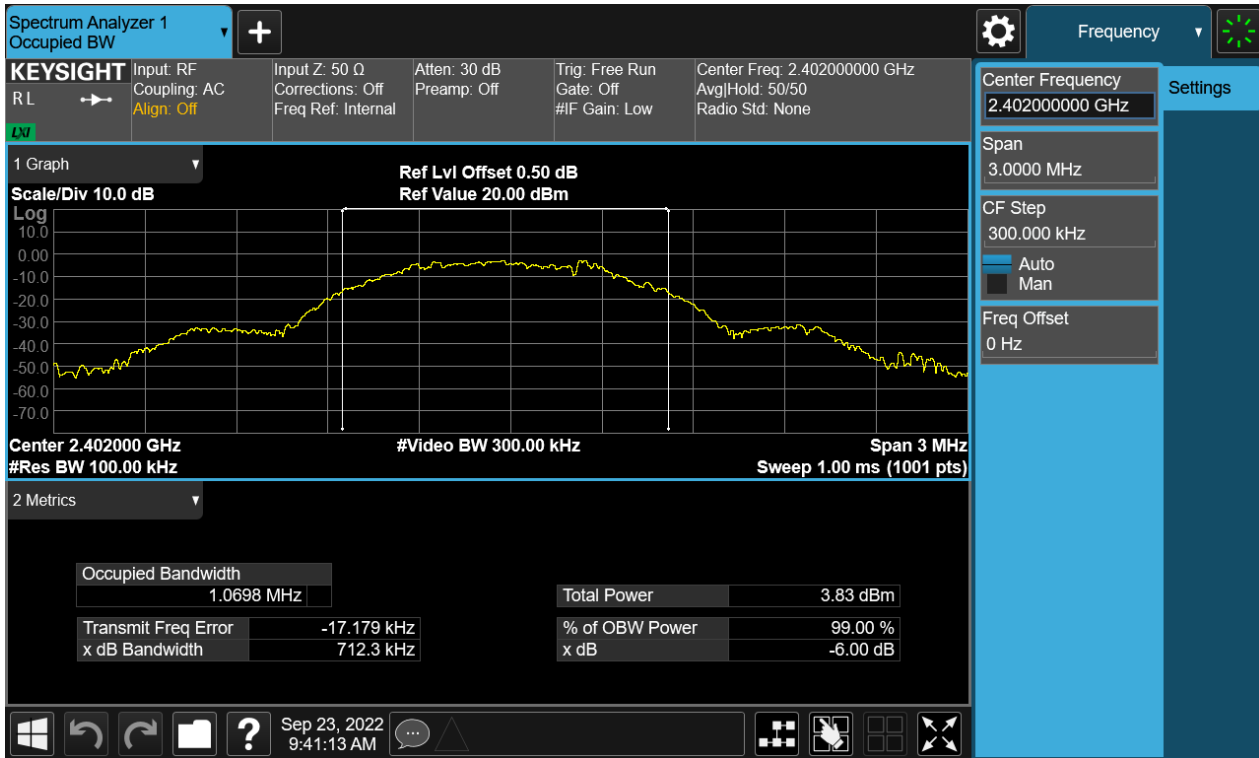
Figure 5: The plots of 99% Bandwidth, 2402MHz
