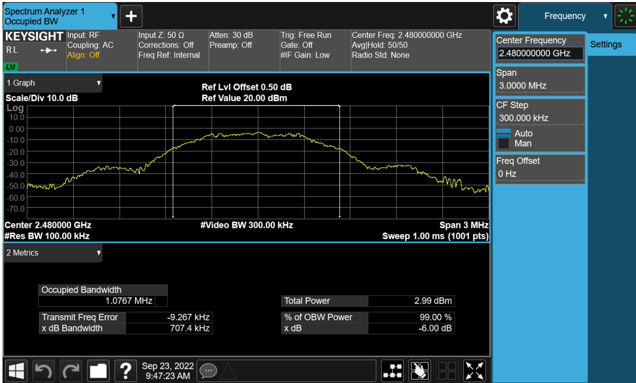
Figure 9: The plots of 99% Bandwidth, 2480MHz
