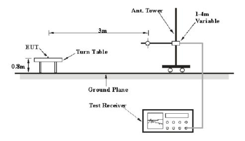
The radiated emission and out of band emission tests were performed in the 3 meters chamber test site, using the setup accordance with the ANSI C63.10-2013. The specification used was the FCC 15.209/15.205 and FCC 15.249 limits.
