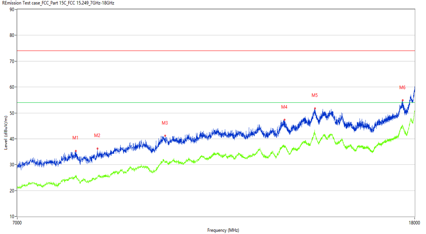
Figure 12: Test plots of Field strength of harmonics, 2403MHz, 7GHz-18GHz, Vertical polarization
