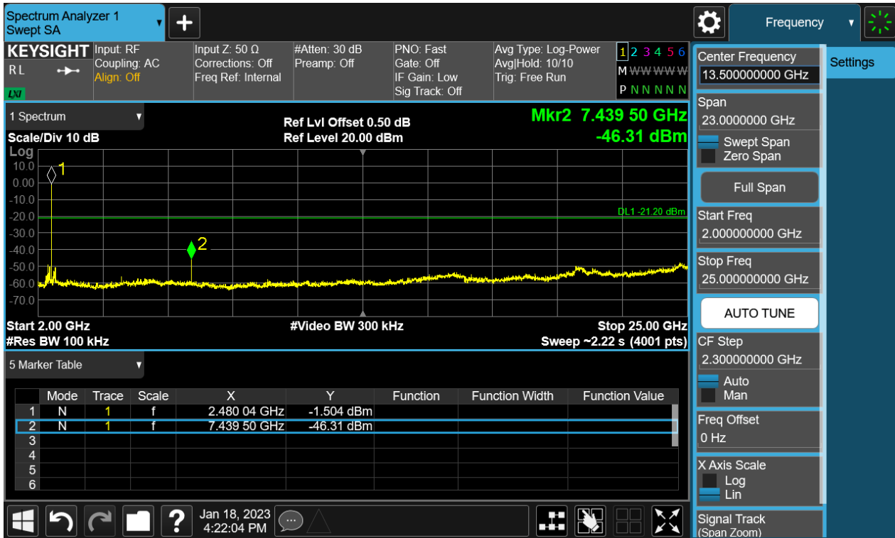
Figure 36: The plots of Conducted Spurious Emission & Authorized-band band-edge, 2402MHz, BLE-2M, Carrier Level
