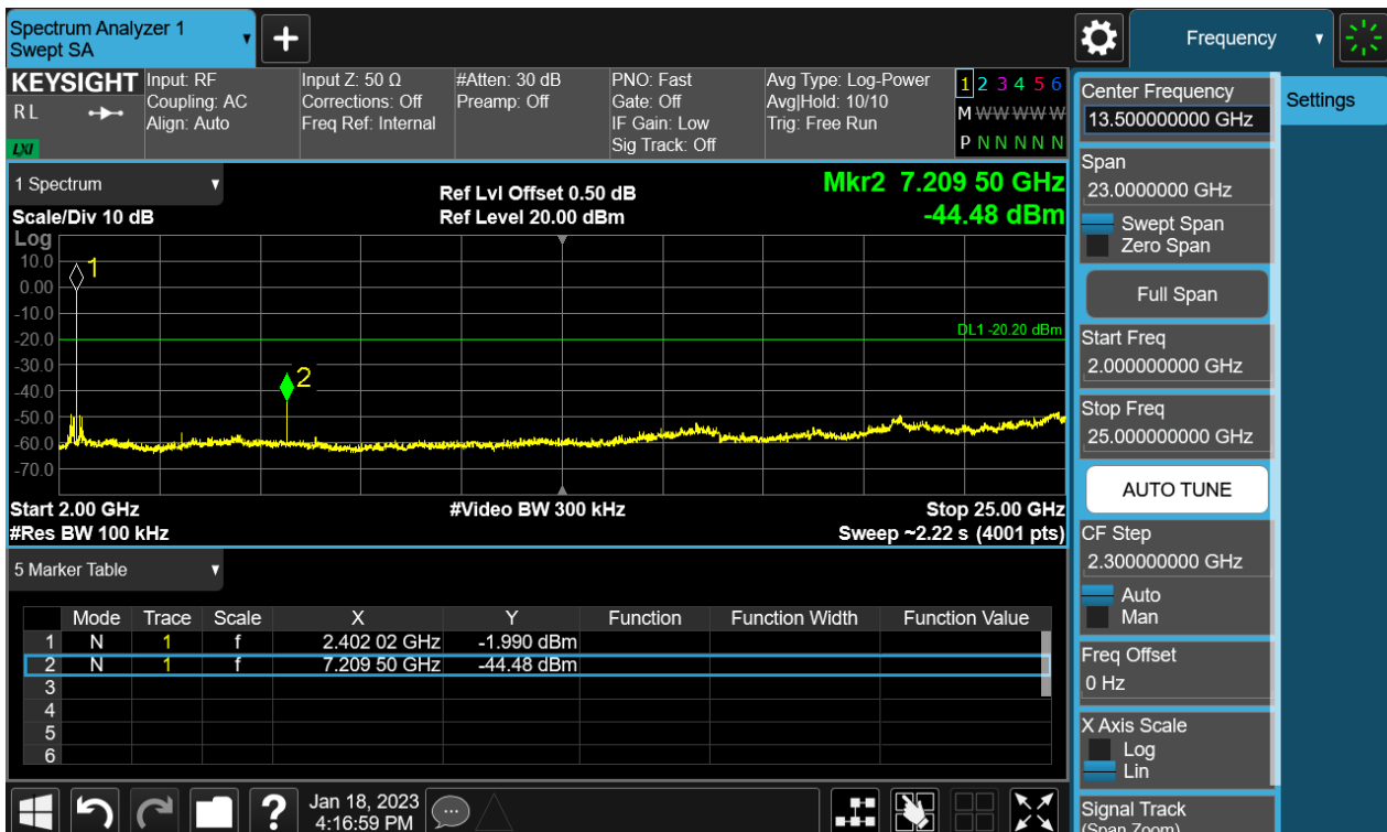
Figure 28: The plots of Conducted Spurious Emission & Authorized-band band-edge, 2402MHz, BLE-1M, Conducted spurious emissions 2GHz-25GHz
