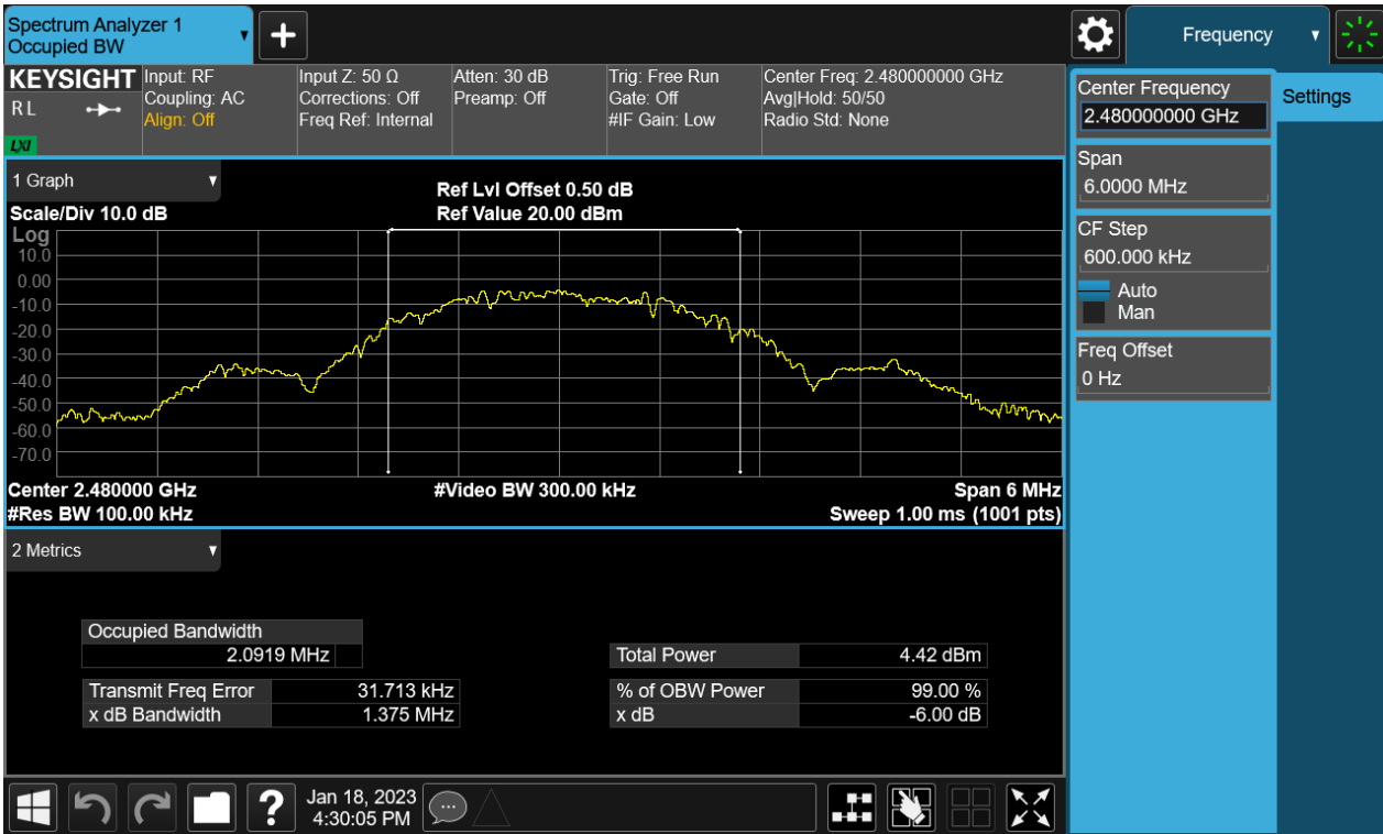
Figure 18: The plots of 99% Bandwidth, 2480MHz, BLE-2M
