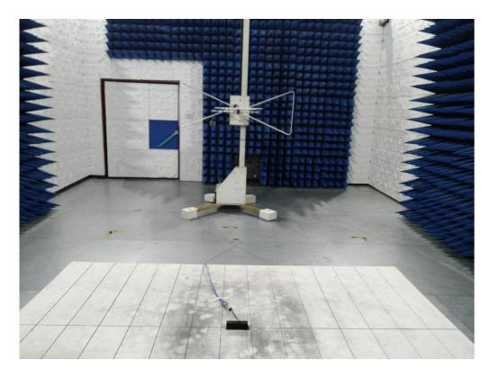
RADIATED EMISSION TEST SETUP ABOVE 1GHZ
