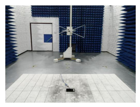
RADIATED EMISSION TEST SETUP ABOVE 1GHZ
