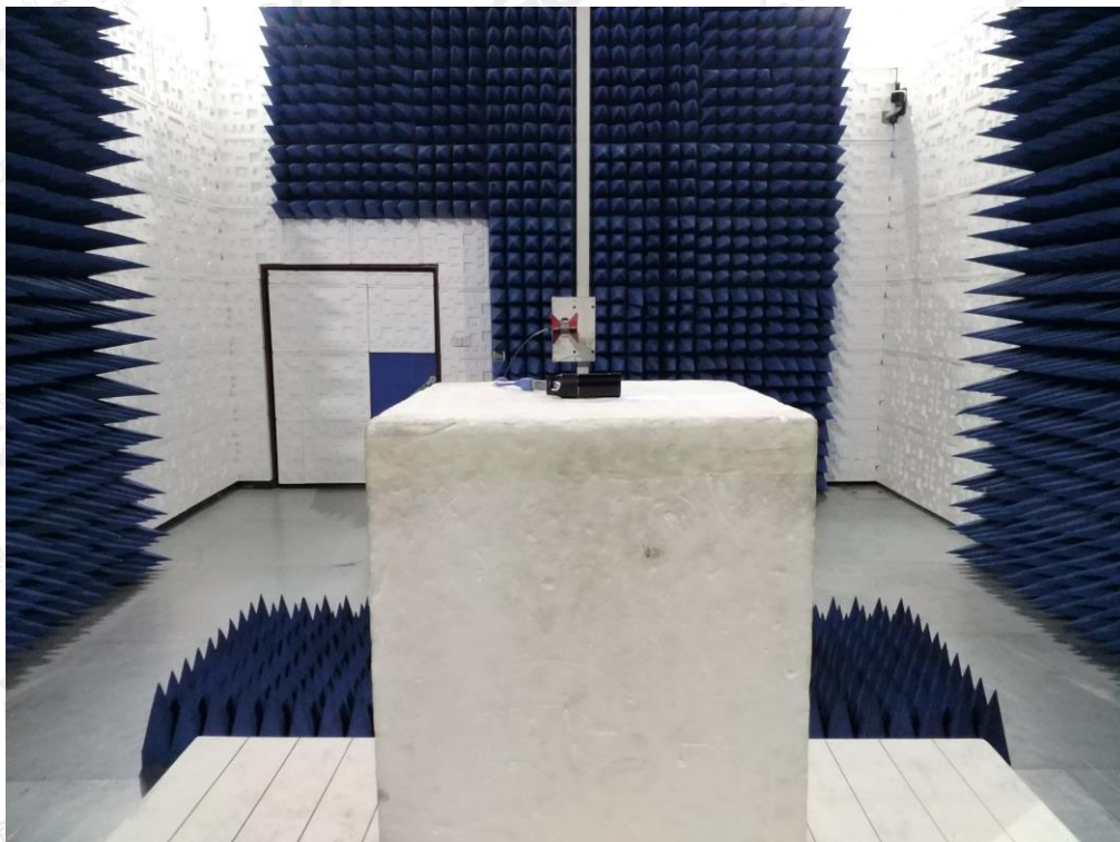
RADIATED EMISSION TEST SETUP ABOVE 1GHZ
