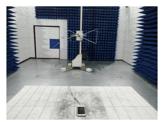
RADIATED EMISSION TEST SETUP ABOVE 1GHZ
