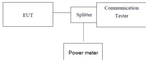
*Note: Measurement setup for testing on Antenna connector*
