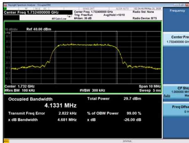
(Plot G2: WCDMA 1700 MHz Channel = 1412 bandwidth)
