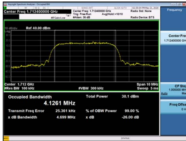
(Plot G1: WCDMA 1700MHz Channel = 1312 bandwidth)
