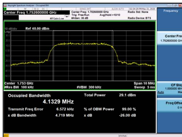
(Plot G2: WCDMA 1700 MHz Channel = 1513 bandwidth)
