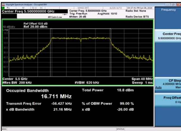
U-NII-2c 26dB Bandwidth-802.11a(20MHz),5700MHz
