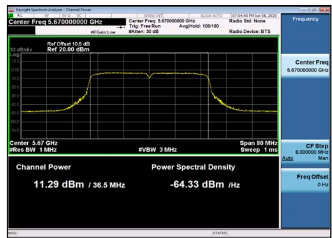
U-NII-2c Output Power-802.11a(20MHz) ,5600MHz
