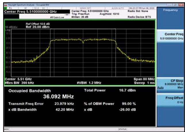
U-NII-2c 26dB Bandwidth-802.11n(40MHz ) ,5510MHz
