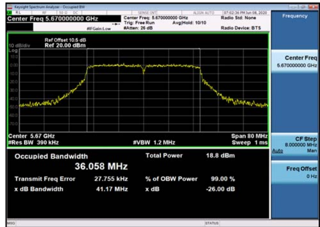
U-NII-2c 26dB Bandwidth-802.11a(20MHz),5600MHz
