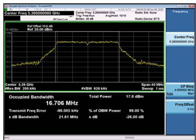
U-NII-2a 26dB Bandwidth-802.11a(20MHz),5260MHz
