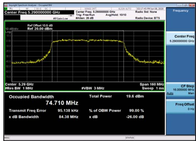
U-NII-2c 26dB Bandwidth-802.11n(20MHz ) ,5600MHz
