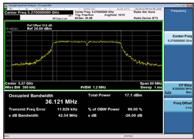
U-NII-2a 26dB Bandwidth-802.11a(20MHz),5260MHz
