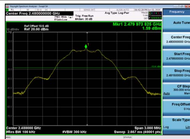
,Plot ,2 Conducted Emission: 2440 ,Band Edge
