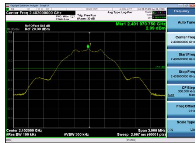
,Plot ,1 Transmitter Spurious Emission : 2480,Referecy Level
