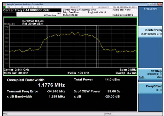
20dB Bandwidth: 8DPSK,2441MHz,3DH5
