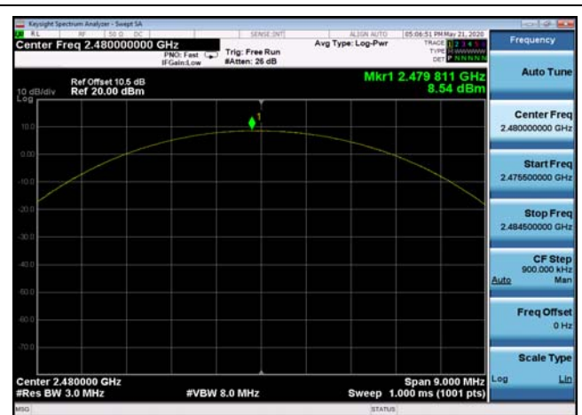
Output Power: DQPSK,2480MHz,2DH5
