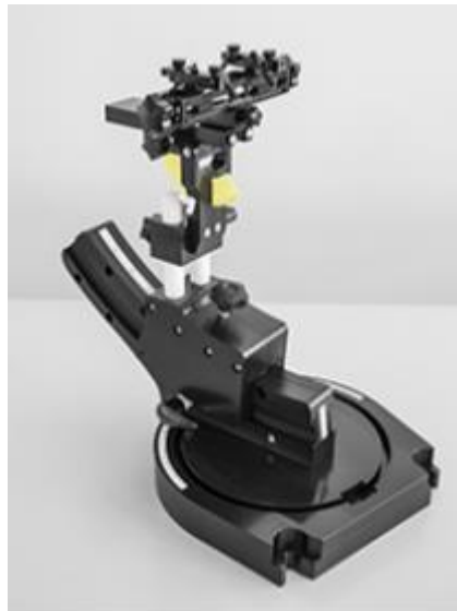
Device holder supplied by SPEAG
