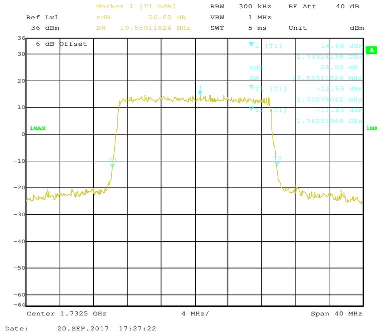
**QPSK (1.4 MHz) - 99% Occupied Bandwidth, Middle channel**
