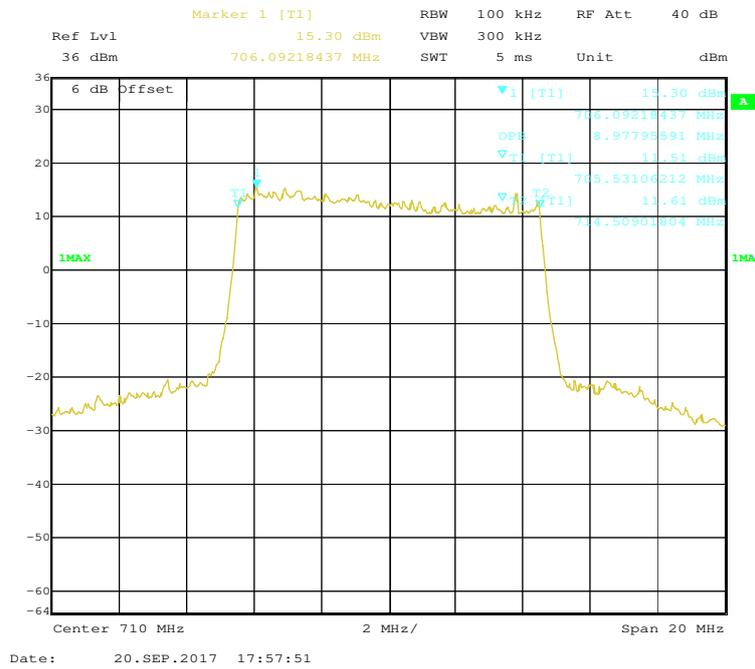
**§ 2.1051; § 22.917 (a);§ 24.238 (a); §27.53 (h)(m) SPURIOUS EMISSIONS AT ANTENNA TERMINALS**
