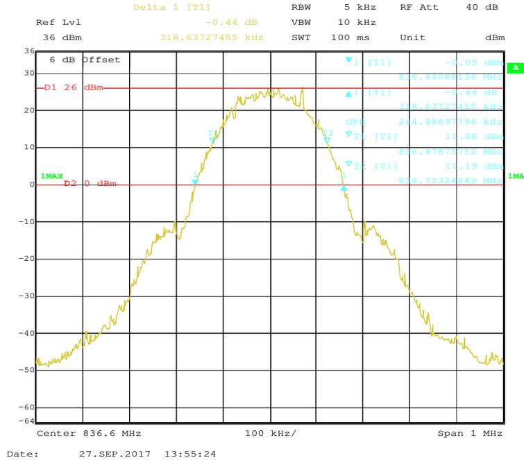
**99% Occupied & 26 dB Emissions Bandwidth for GPRS (GMSK) Mode**
