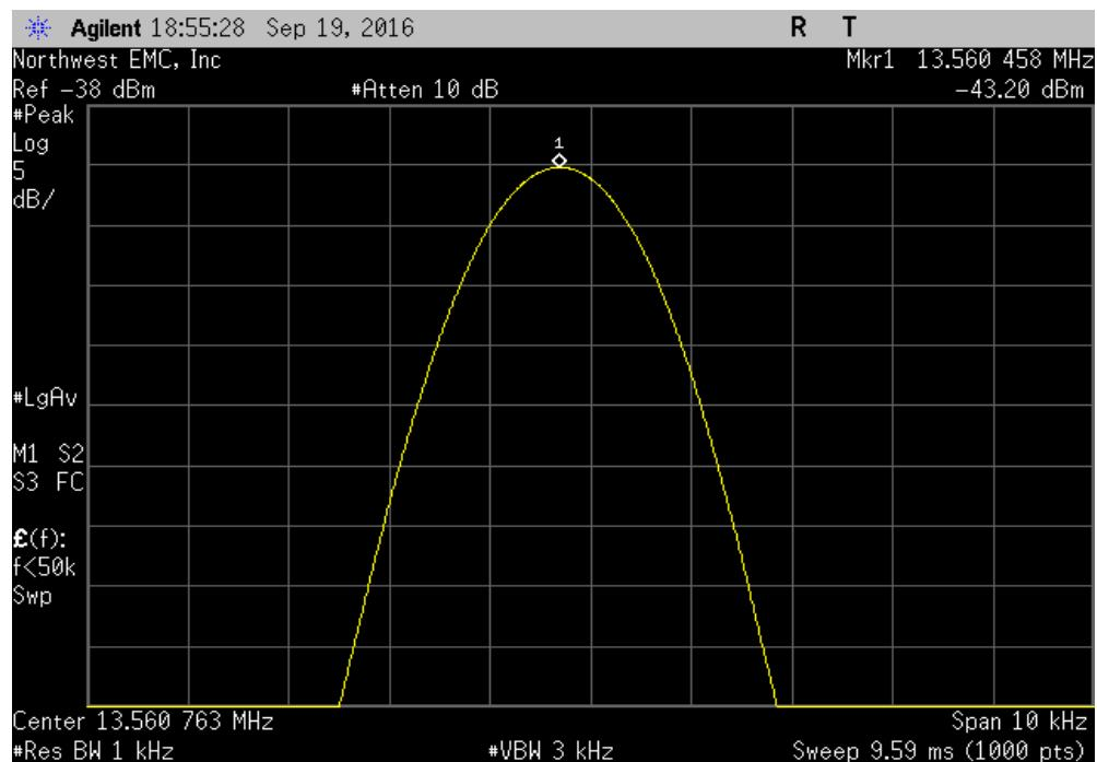
RFID, 13.56 MHz, Temperature: +40°, Startup
