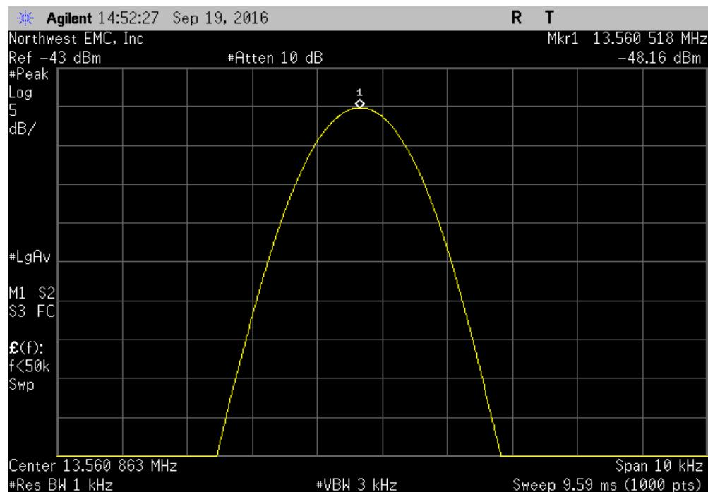
RFID, 13.56 MHz, Temperature: +10°, After 5 Minutes
