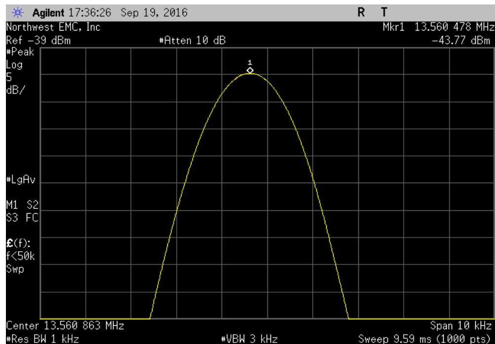
RFID, 13.56 MHz, Temperature: +30°, After 5 Minutes
