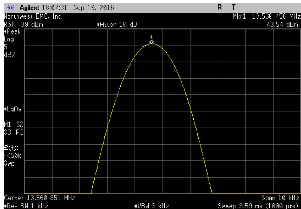
RFID, 13.56 MHz, Temperature: +40°, After 5 Minutes
