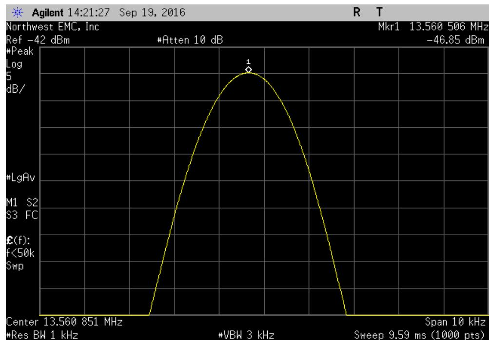
RFID, 13.56 MHz, Temperature: +20°, After 5 Minutes
