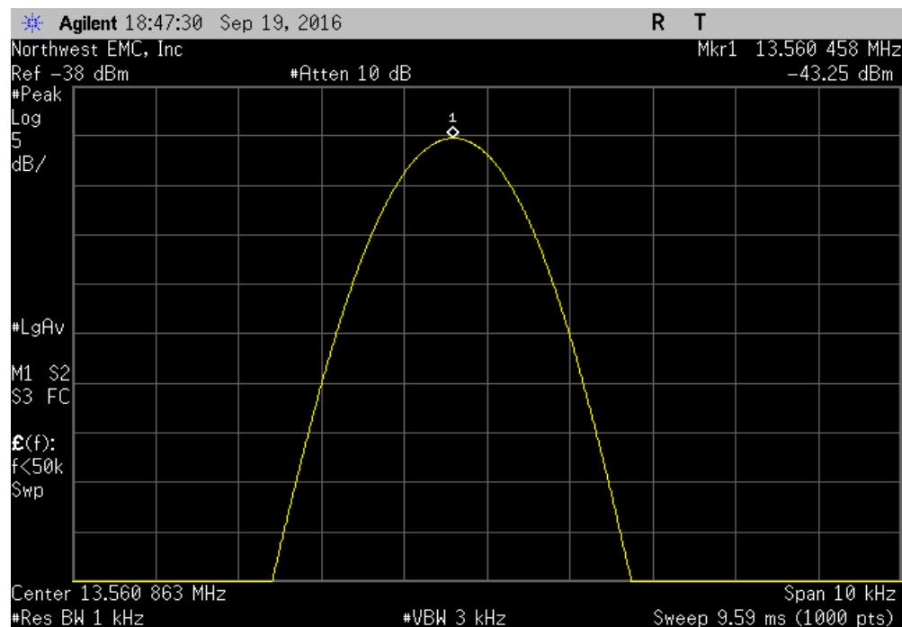
RFID, 13.56 MHz, Temperature: +50°, After 5 Minutes
