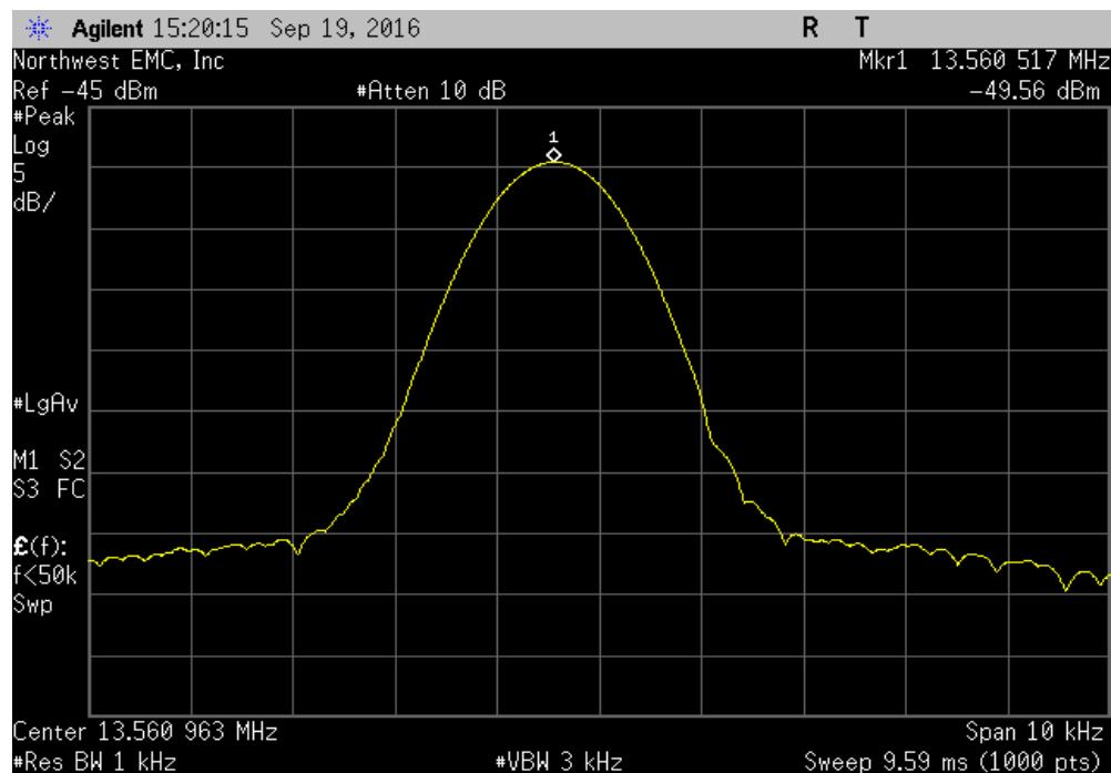
RFID, 13.56 MHz, Temperature: 0°, After 5 Minutes
