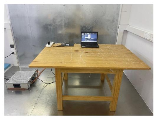
1.2 Set-up for Conducted RF test at Antenna Port
