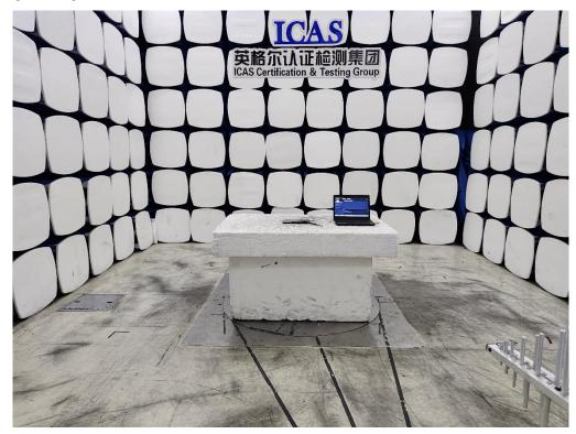
1.3 Set-up for Spurious Emissions below 1GHz
