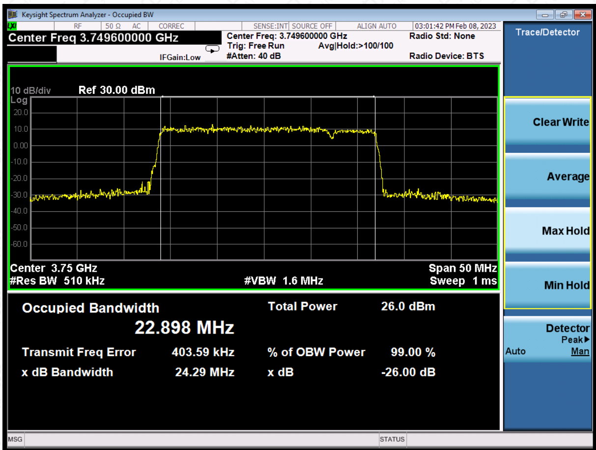
LTE CA band 43Part27 , 20MHz+5MHz Bandwidth,16QAM (99% BW)
