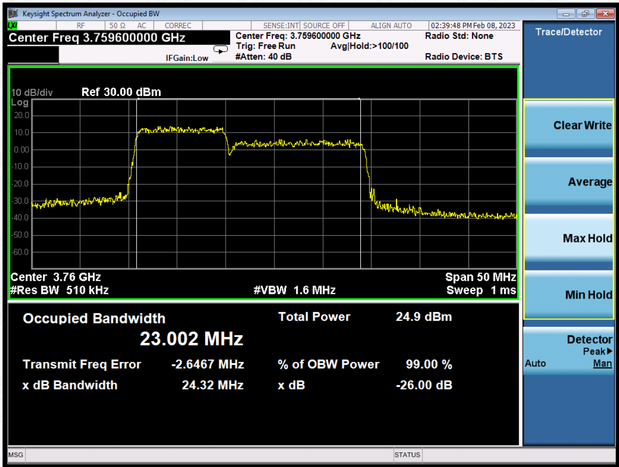
LTE CA band 43Part27 , 10MHz+15MHz Bandwidth,64QAM (99% BW)
