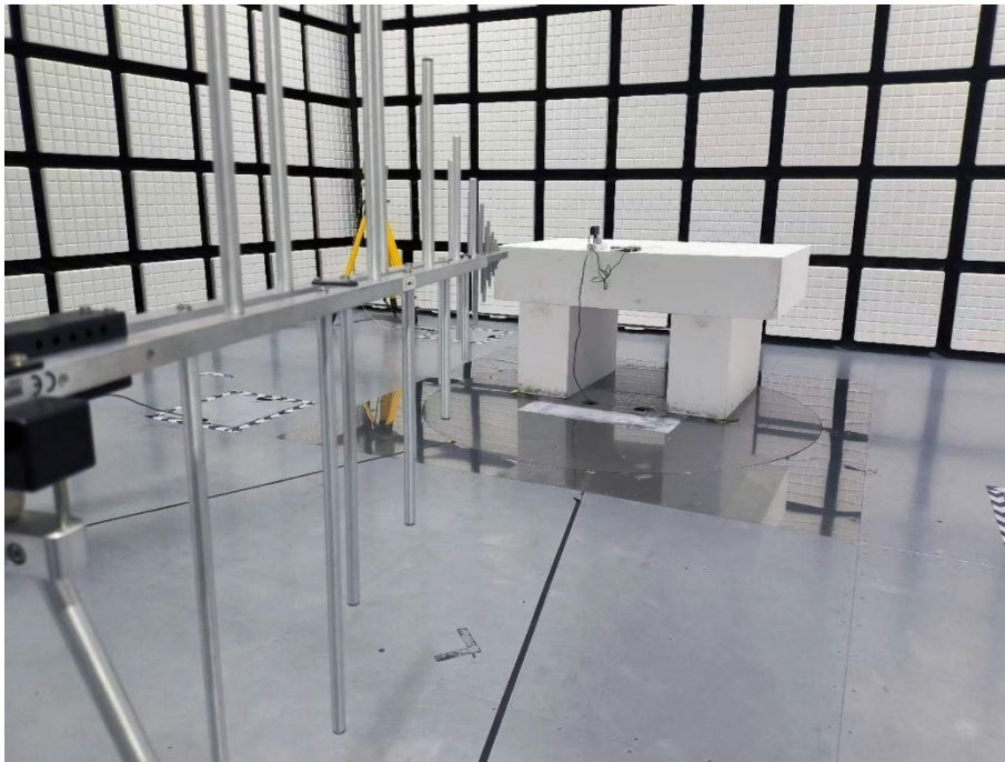
Description: Back view of Radiated Emission Test Setup (Below 1GHz)
