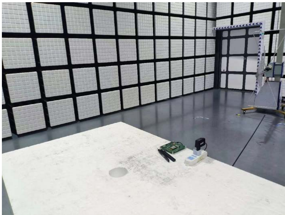
Description: Back view of Radiated Emission Test Setup (Below 1GHz)
