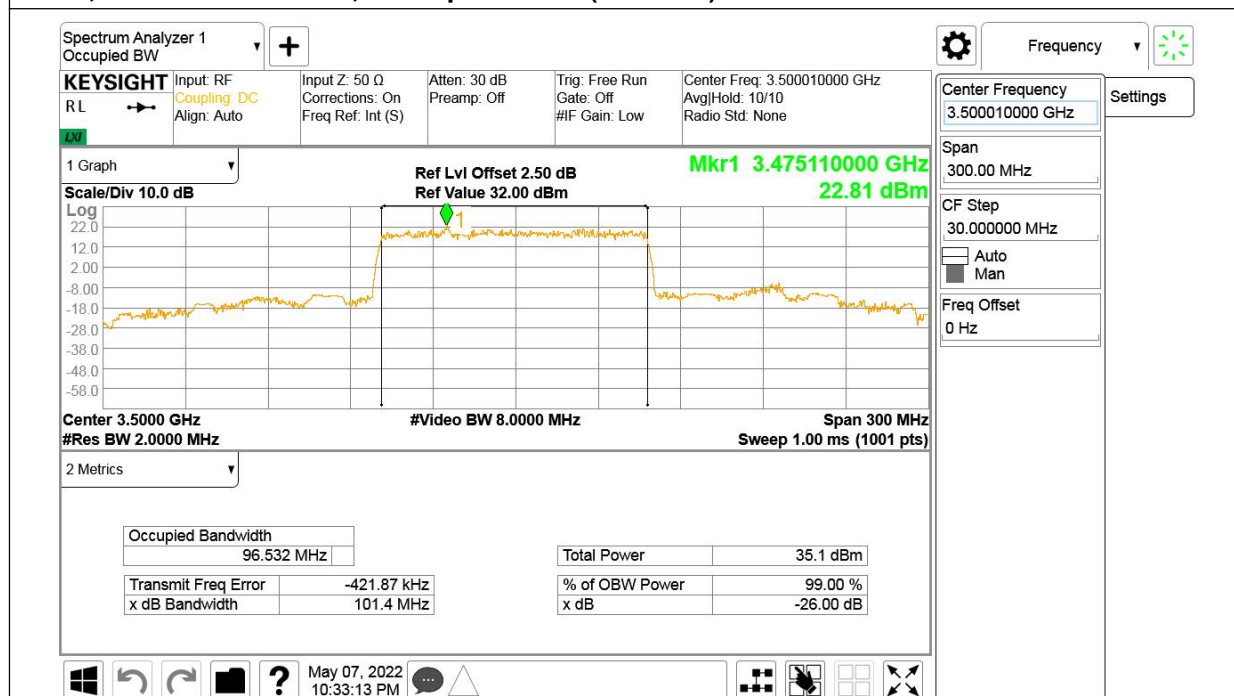
n77L,100MHz Bandwidth,DFT-s-QPSK (99% BW)
