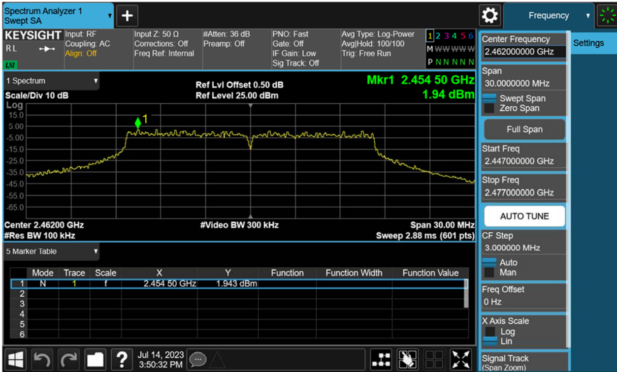
Figure 30: Conducted Spurious Emission & Authorized-band band-edge, 802.11g, 2462MHz Carrier Level
