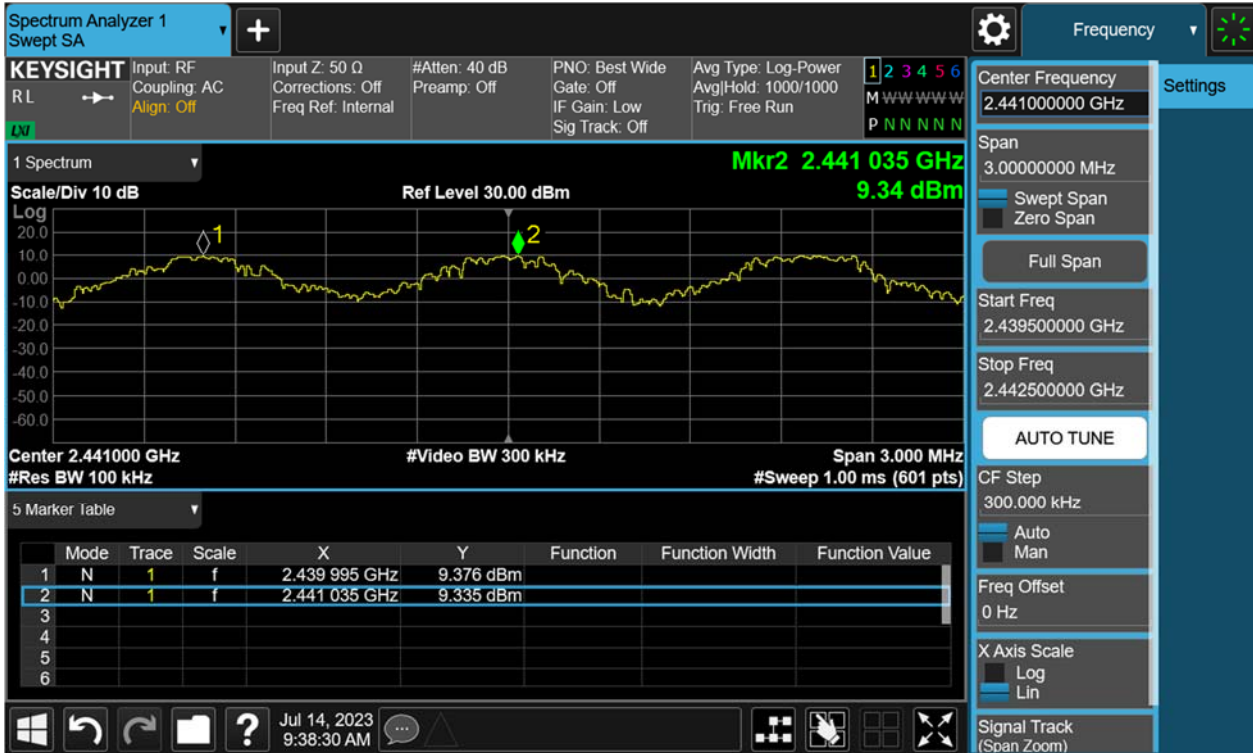
Figure 32: Hopping Frequency Separation, Hopping Mode, \pi/4 -DQPSK
