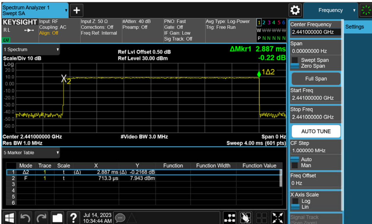
Figure 42: Time of Occupancy, 2441MHz, \pi/4 -DQPSK DH5
