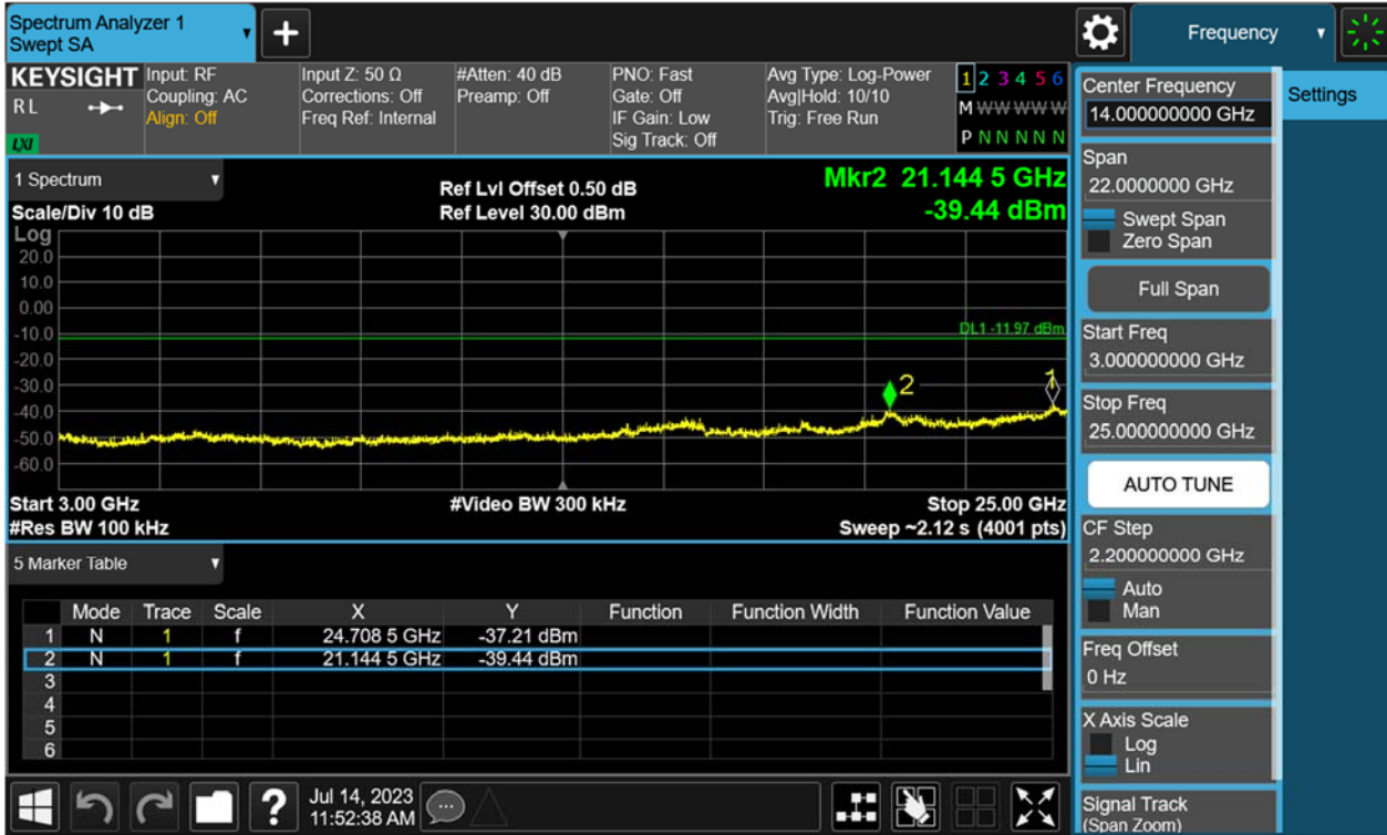
Figure 28: Conducted Spurious Emission & Authorized-band band-edge, Hopping Mode, GFSK Carrier Level
