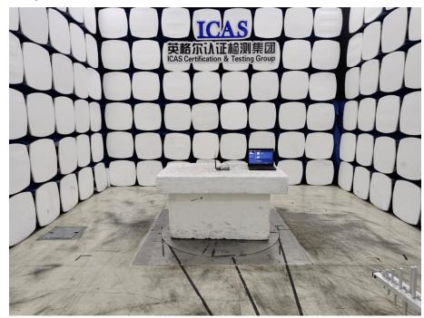
1.3 Set-up for Spurious Emissions below 1GHz
