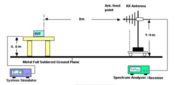
For radiated test from above 1GHz
