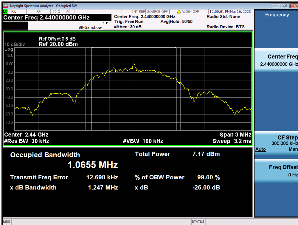
Figure 7: The plots of 99% Bandwidth, 2440MHz, BLE
