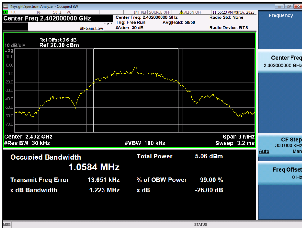
Figure 5: The plots of 99% Bandwidth, 2402MHz, BLE
