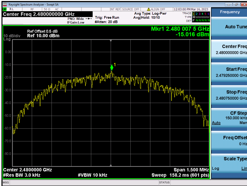
Figure 12: The plots of Power Spectral Density, 2480MHz, BLE
