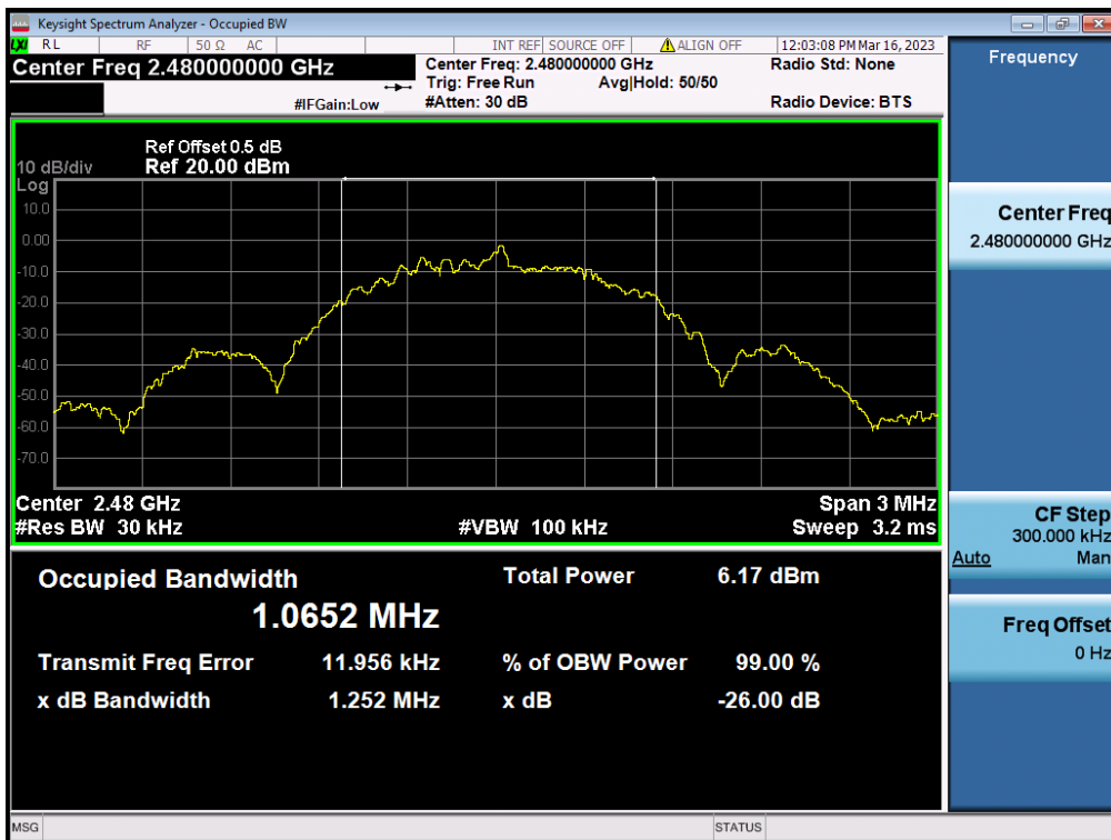
Figure 9: The plots of 99% Bandwidth, 2480MHz, BLE
