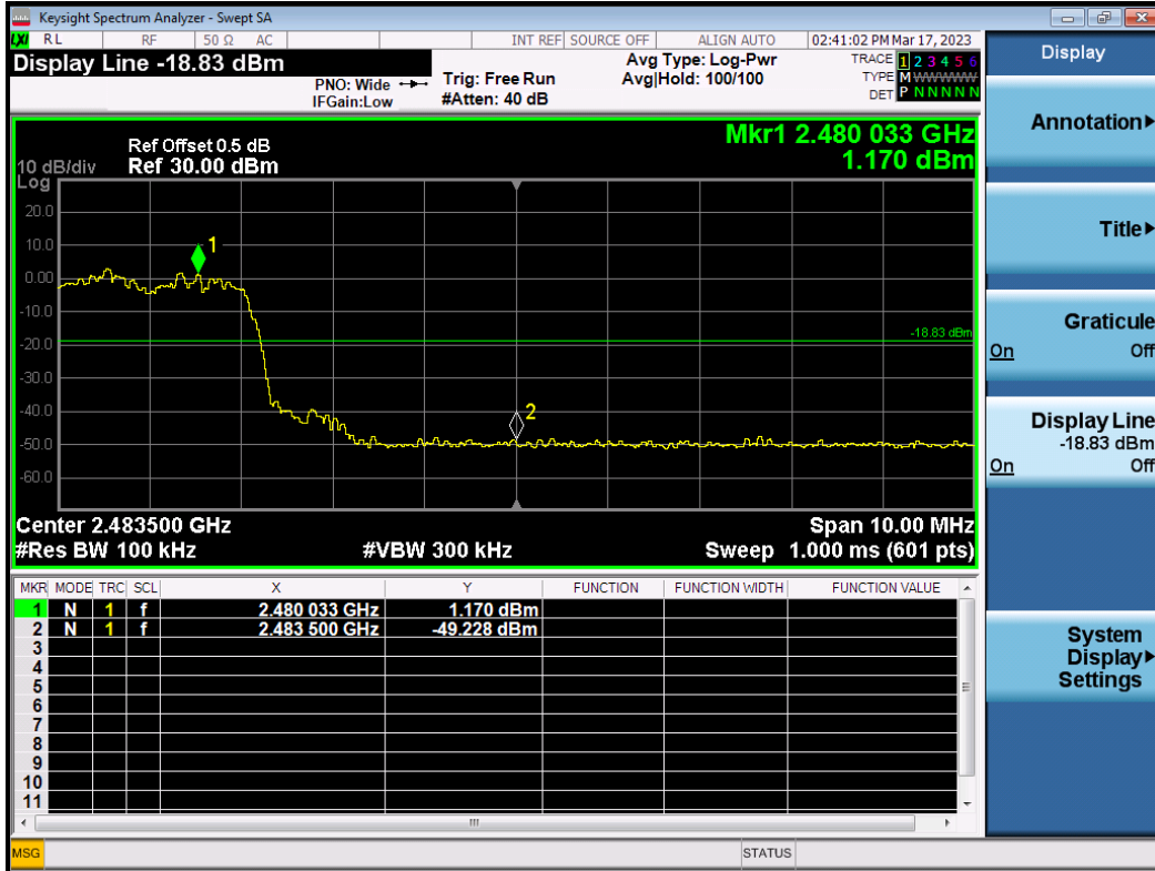
Figure 60: The plots of Conducted Spurious Emission & Authorized-band band-edge, Hopping Mode, \pi/4 -DQPSK, Conducted spurious emissions 30MHz-3GHz
