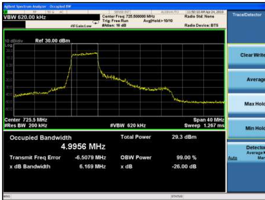
LTE Band28 16QAM 99% Channel 27435 BW=20MHz RB=27 RB Offset=0
