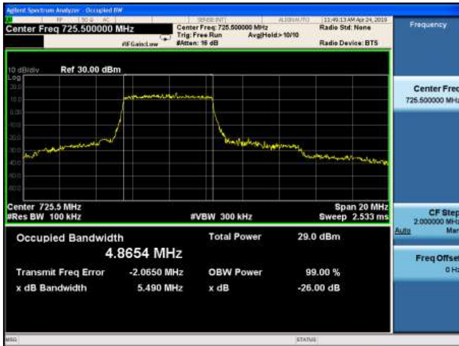
LTE Band28 16QAM 99% Channel 27435 BW=10MHz RB=27 RB Offset=0
