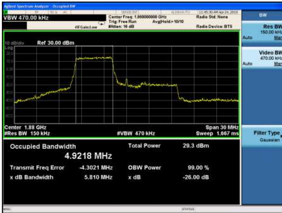
LTE Band2 16QAM 99% Channel 18900 BW=15MHz RB=27 RB Offset=0
