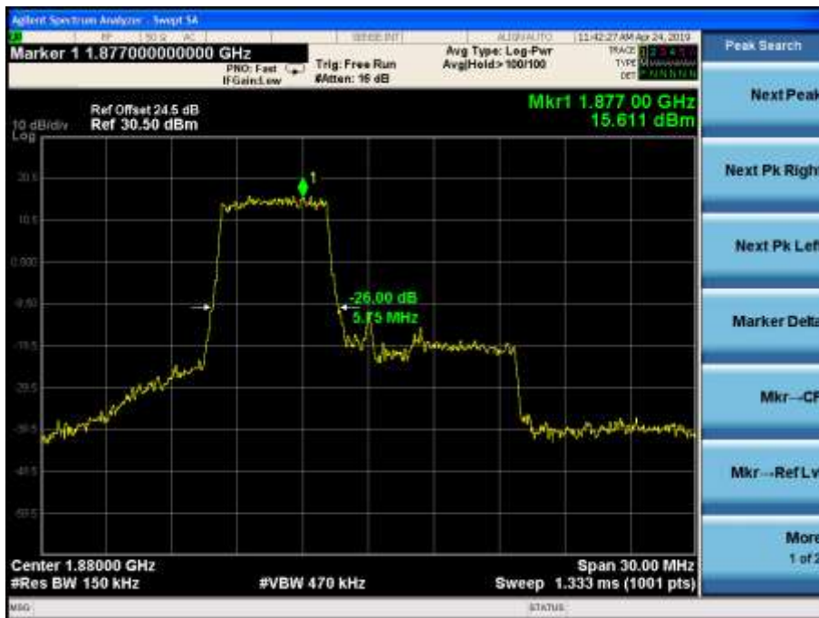
LTE Band2 16QAM -26dBc Channel 18900 BW=15MHz RB=27 RB Offset=0
