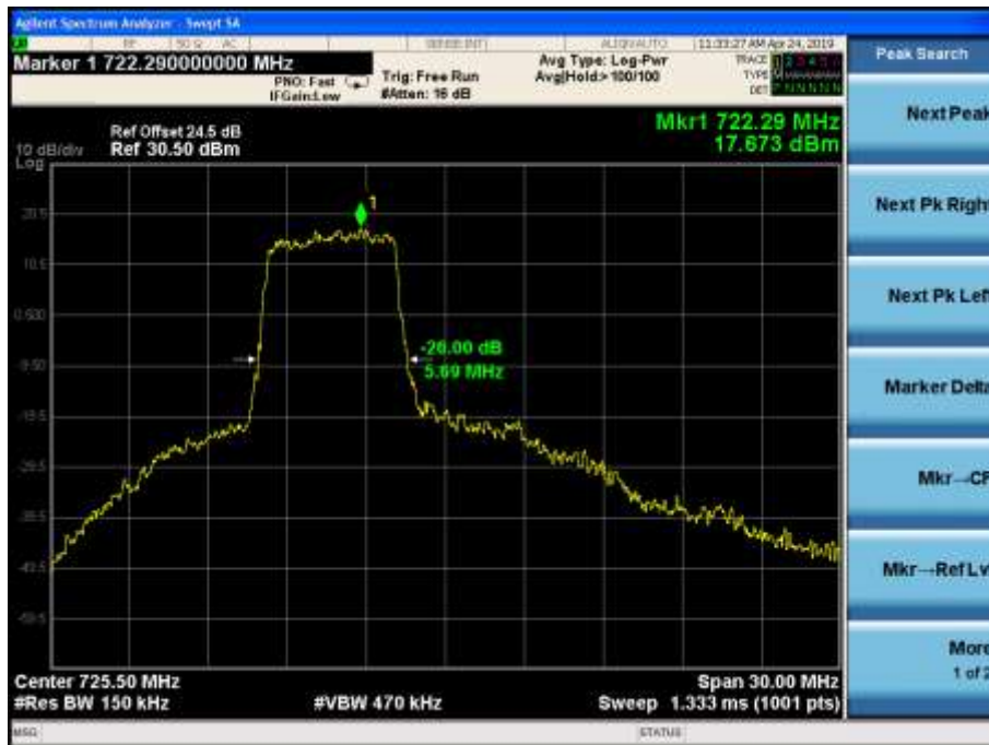
LTE Band28 16QAM -26dBc Channel 27435 BW=15MHz RB=27 RB Offset=0
