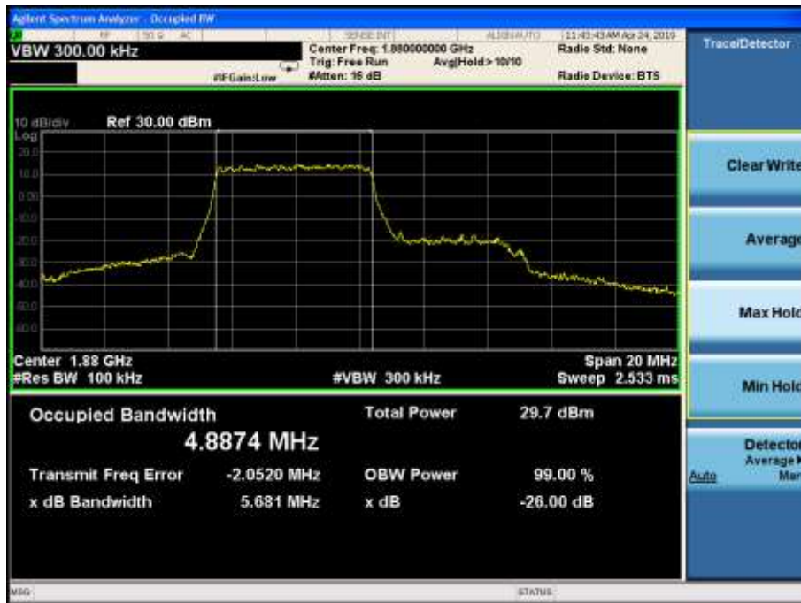
LTE Band2 16QAM 99% Channel 18900 BW=10MHz RB=27 RB Offset=0
