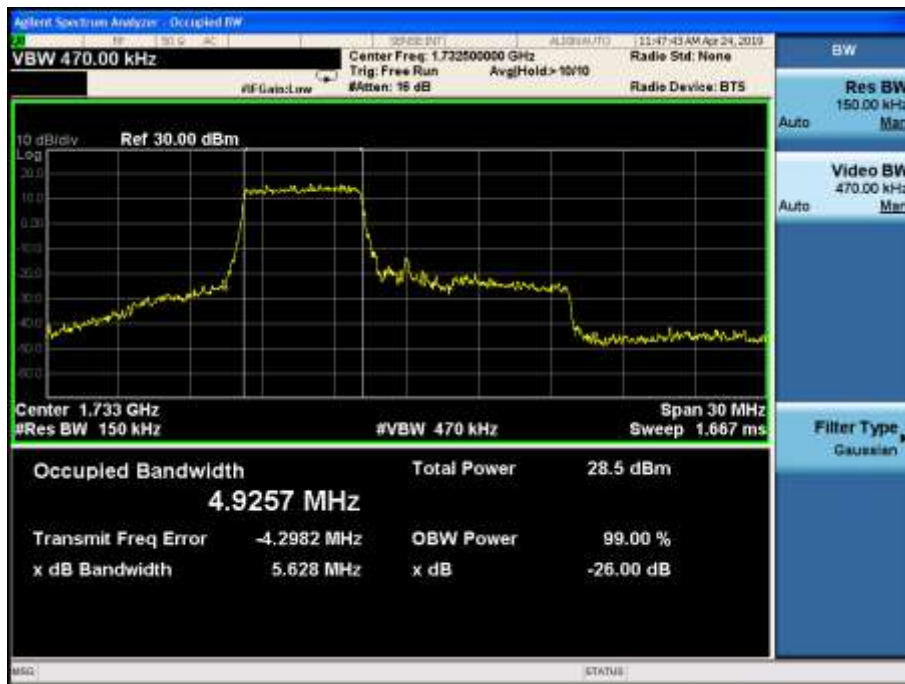
LTE Band4 16QAM 99% Channel 20175 BW=15MHz RB=27 RB Offset=0
