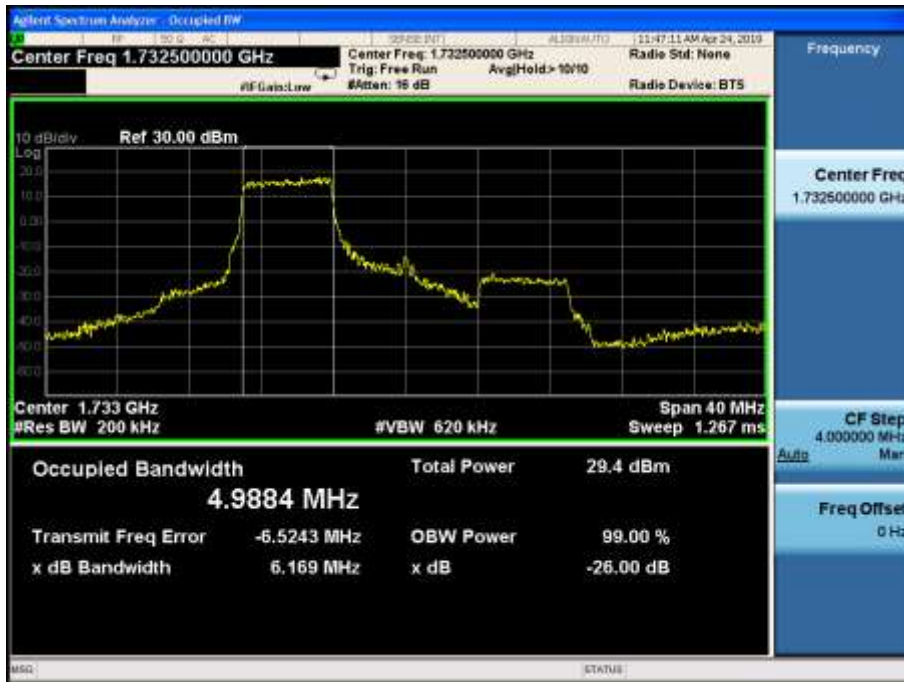
LTE Band4 16QAM 99% Channel 20175 BW=20MHz RB=27 RB Offset=0
