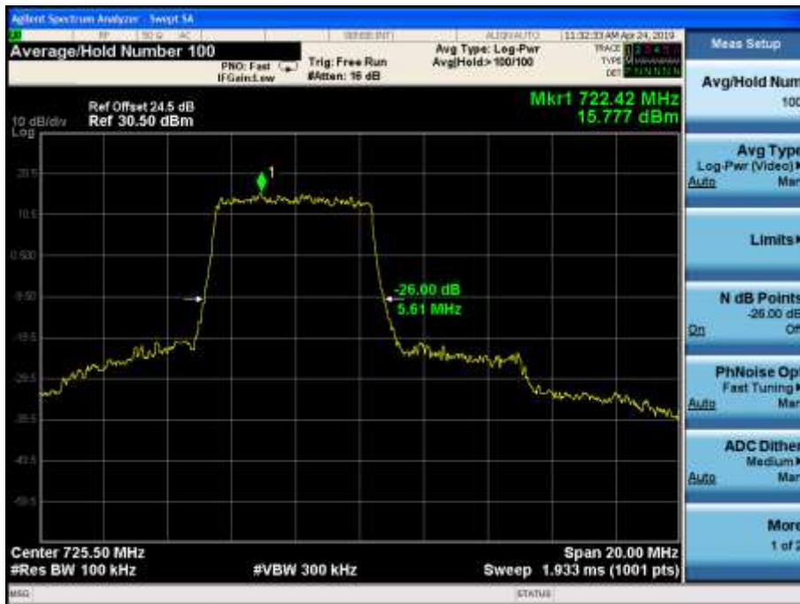
LTE Band28 16QAM -26dBc Channel 27435 BW=10MHz RB=27 RB Offset=0
