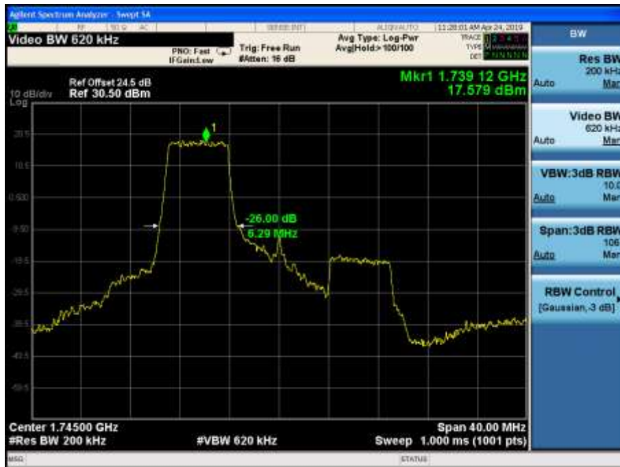
LTE Band66 16QAM -26dBc Channel 132322 BW=20MHz RB=27 RB Offset=0
