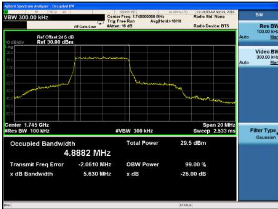
LTE Band66 16QAM -99% Channel 132322 BW=10MHz RB=27 RB Offset=0
