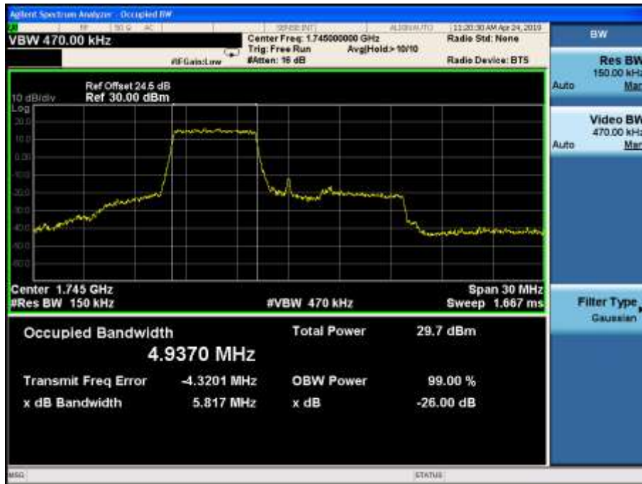
LTE Band66 16QAM 99% Channel 132322 BW=15MHz RB=27 RB Offset=0
