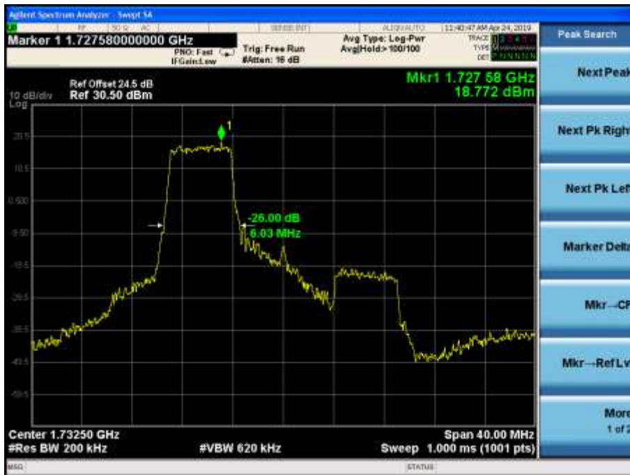
LTE Band4 16QAM -26dBc Channel 20175 BW=20MHz RB=27 RB Offset=0
