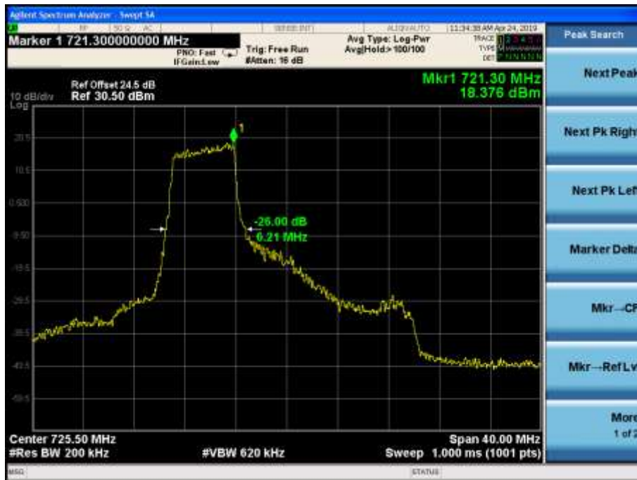
LTE Band28 16QAM -26dBc Channel 27435 BW=20MHz RB=27 RB Offset=0
