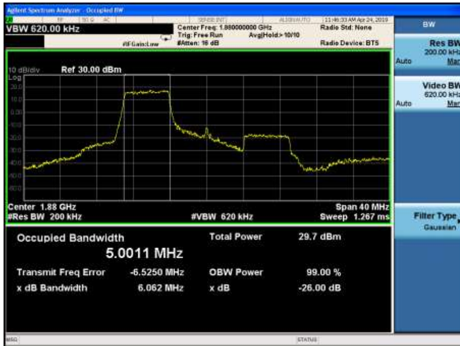
LTE Band2 16QAM 99% Channel 18900 BW=20MHz RB=27 RB Offset=0
