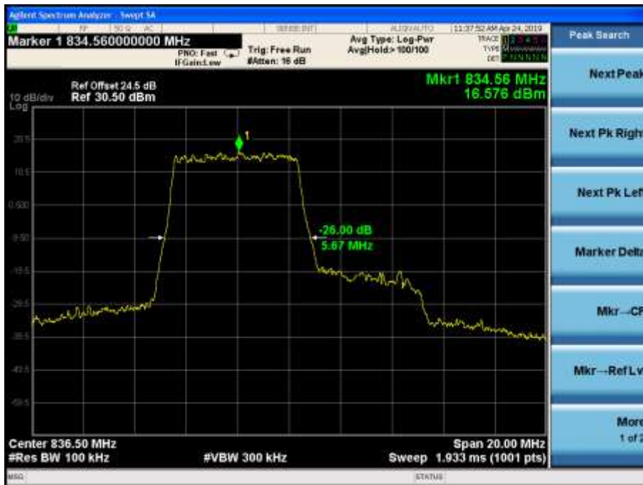
LTE Band5 16QAM -26dBc Channel 20525 BW=10MHz RB=27 RB Offset=0
