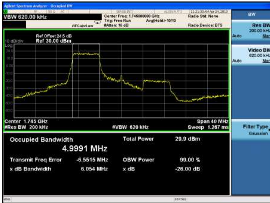
LTE Band66 16QAM 99% Channel 132322 BW=20MHz RB=27 RB Offset=0
