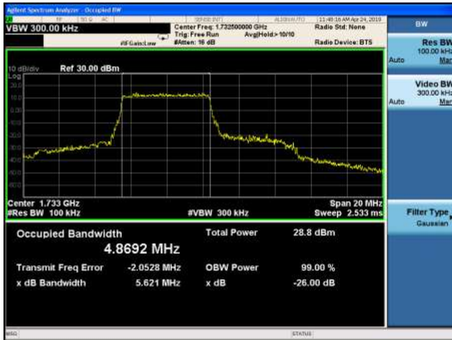
LTE Band4 16QAM 99% Channel 20175 BW=10MHz RB=27 RB Offset=0
