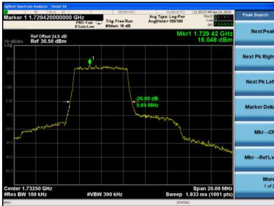
LTE Band4 16QAM -26dBc Channel 20175 BW=10MHz RB=27 RB Offset=0
