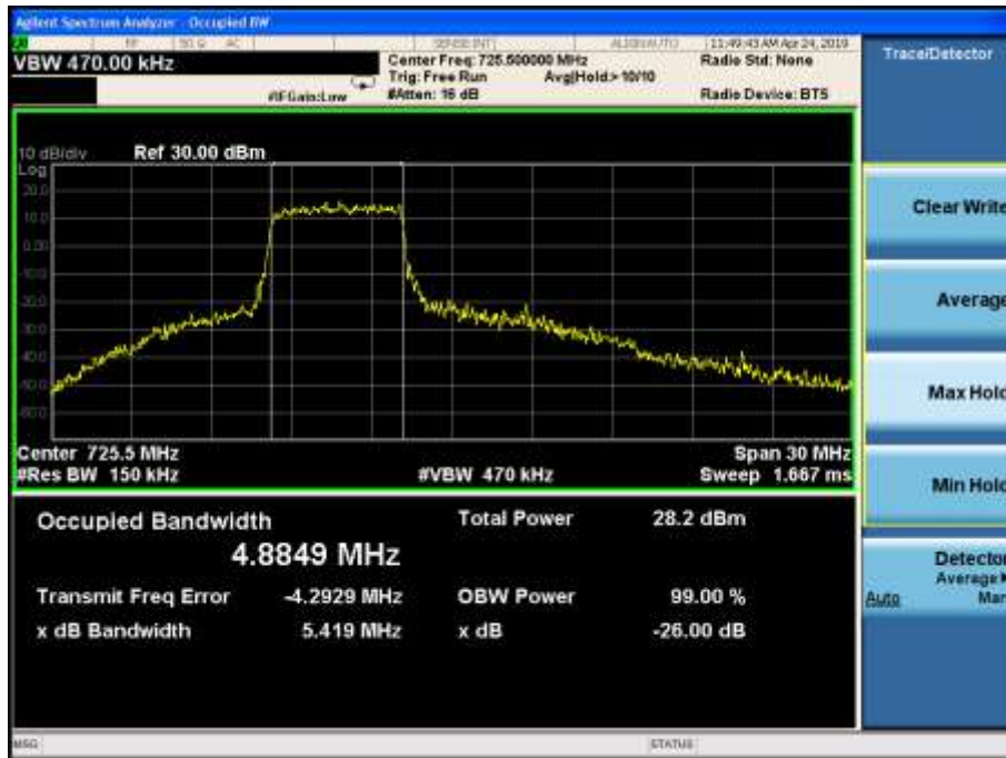
LTE Band28 16QAM 99% Channel 27435 BW=15MHz RB=27 RB Offset=0
