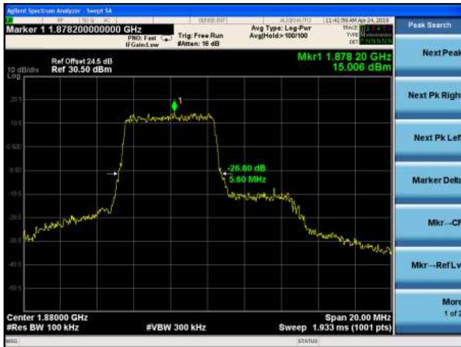
LTE Band2 16QAM -26dBc Channel 18900 BW=10MHz RB=27 RB Offset=0
