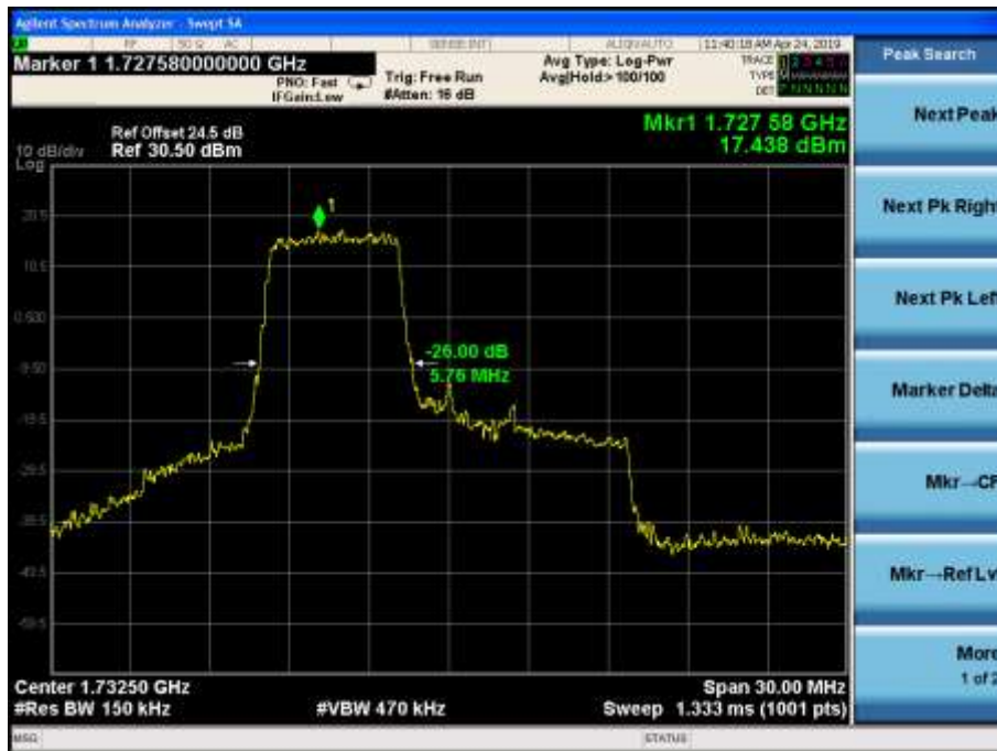
LTE Band4 16QAM -26dBc Channel 20175 BW=15MHz RB=27 RB Offset=0
