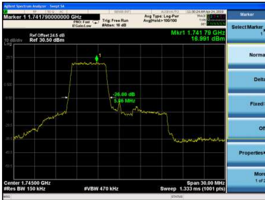
LTE Band66 16QAM -26dBc Channel 132322 BW=15MHz RB=27 RB Offset=0
