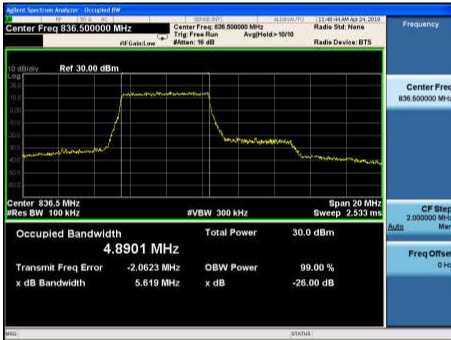
LTE Band5 16QAM 99% Channel 20525 BW=10MHz RB=27 RB Offset=0
