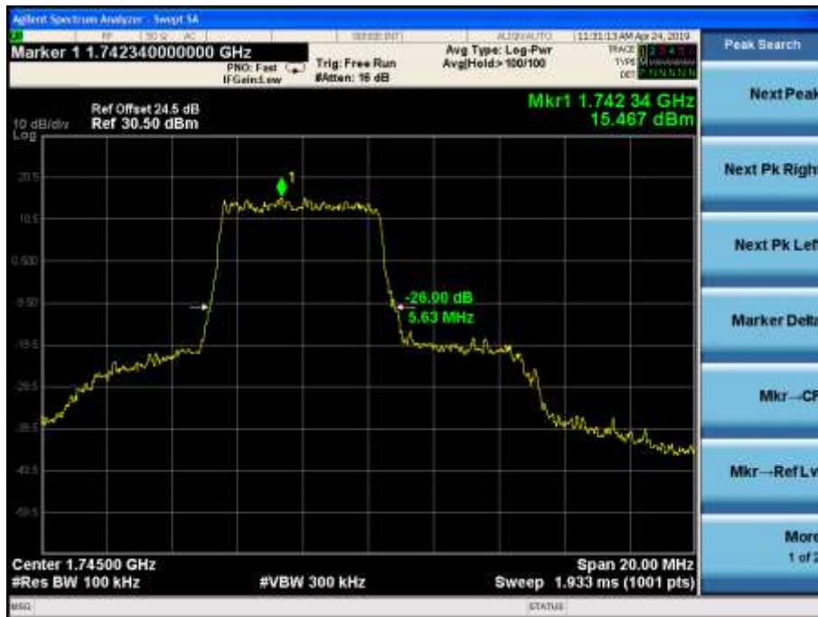
LTE Band66 16QAM -26dBc Channel 132322 BW=10MHz RB=27 RB Offset=0
