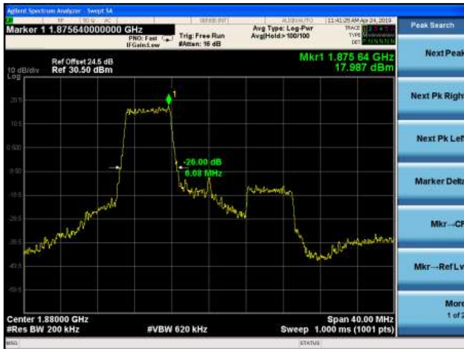
LTE Band2 16QAM -26dBc Channel 18900 BW=20MHz RB=27 RB Offset=0
