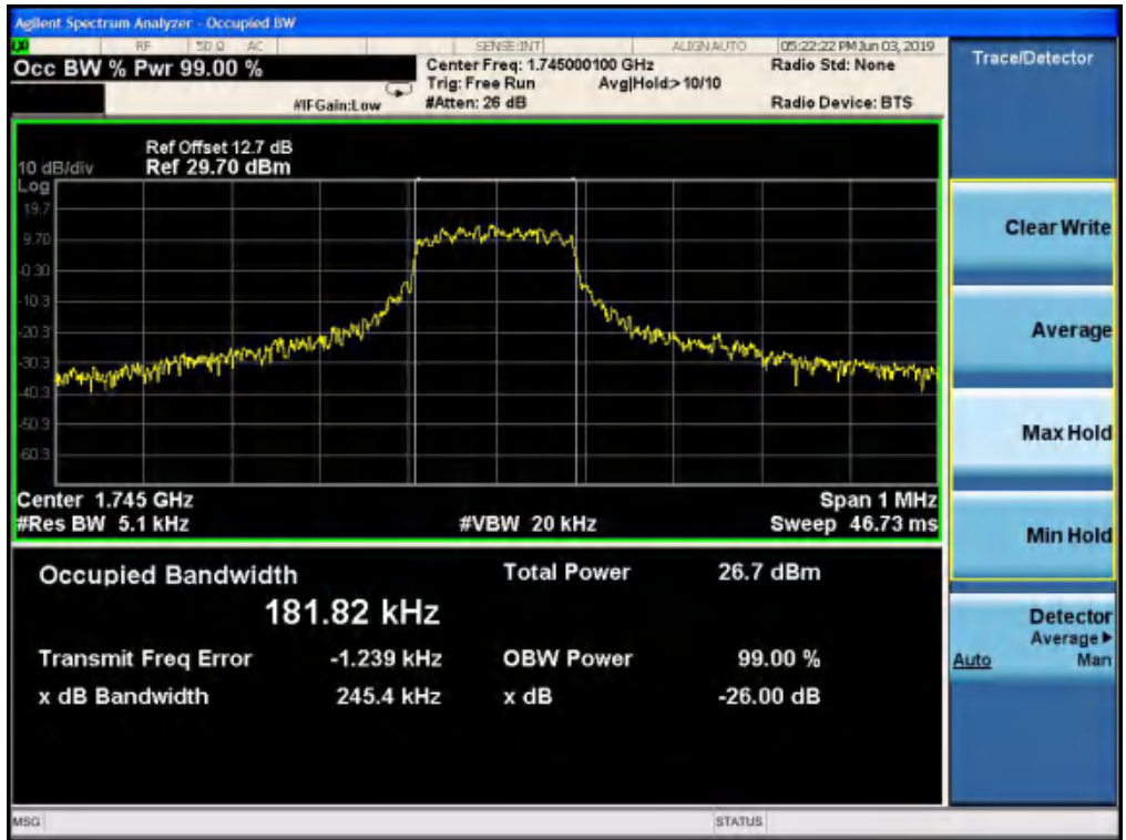
NB-IoT standalone band 66 132322 QPSK(99%)
