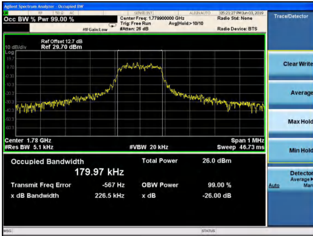
NB-IoT standalone band 66 132671 QPSK(99%)
