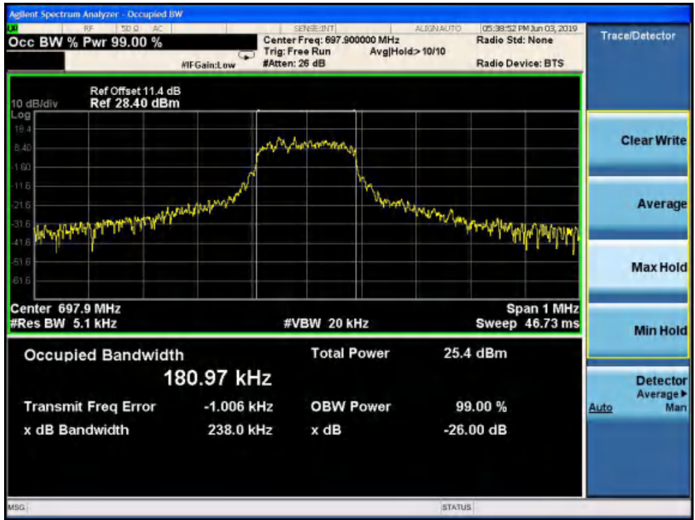
NB-IoT standalone band 71 133471 QPSK(99%)
