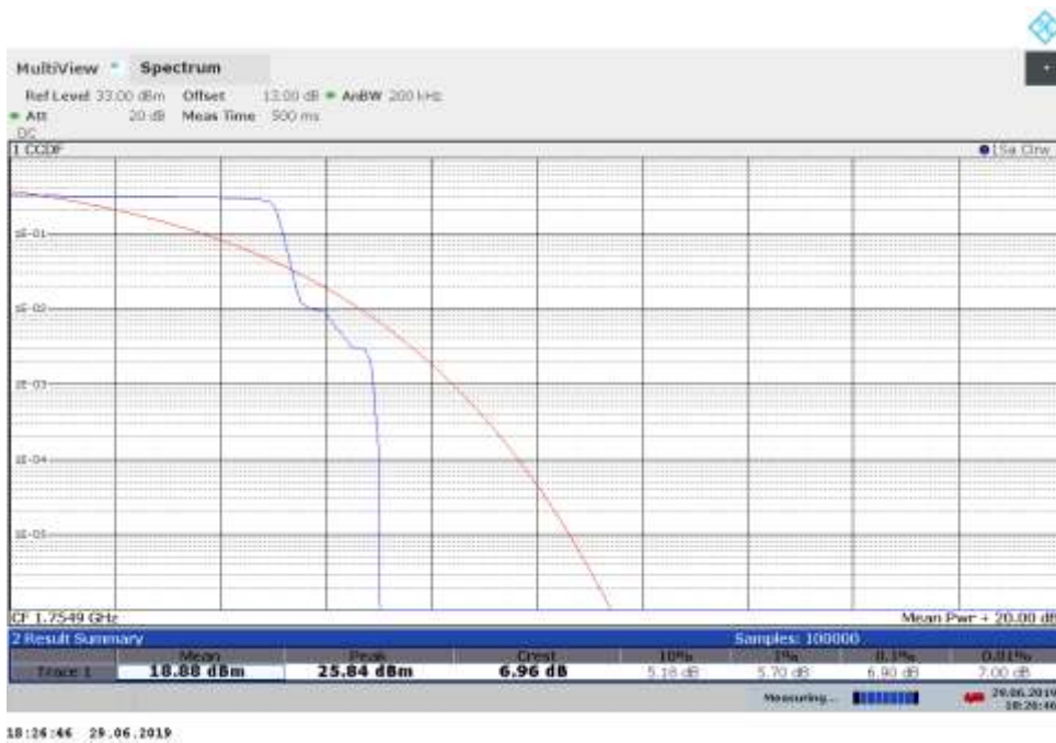
NB-IoT Band 4, High Channel, QPSK, 1
