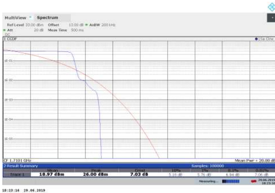
NB-IoT Band 4, Low Channel, QPSK, 1
