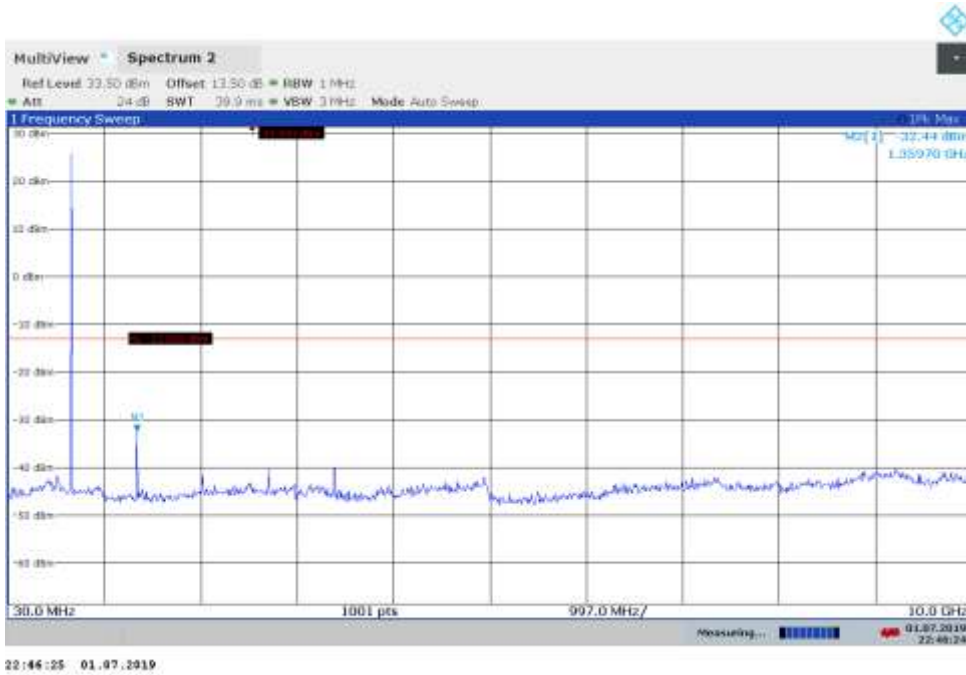
30MHz to 10GHz, Mid Channel, Subcarrier (15kHz), BPSK, 1@0 Note: The strong emission shown in each case is the carrier signal.
