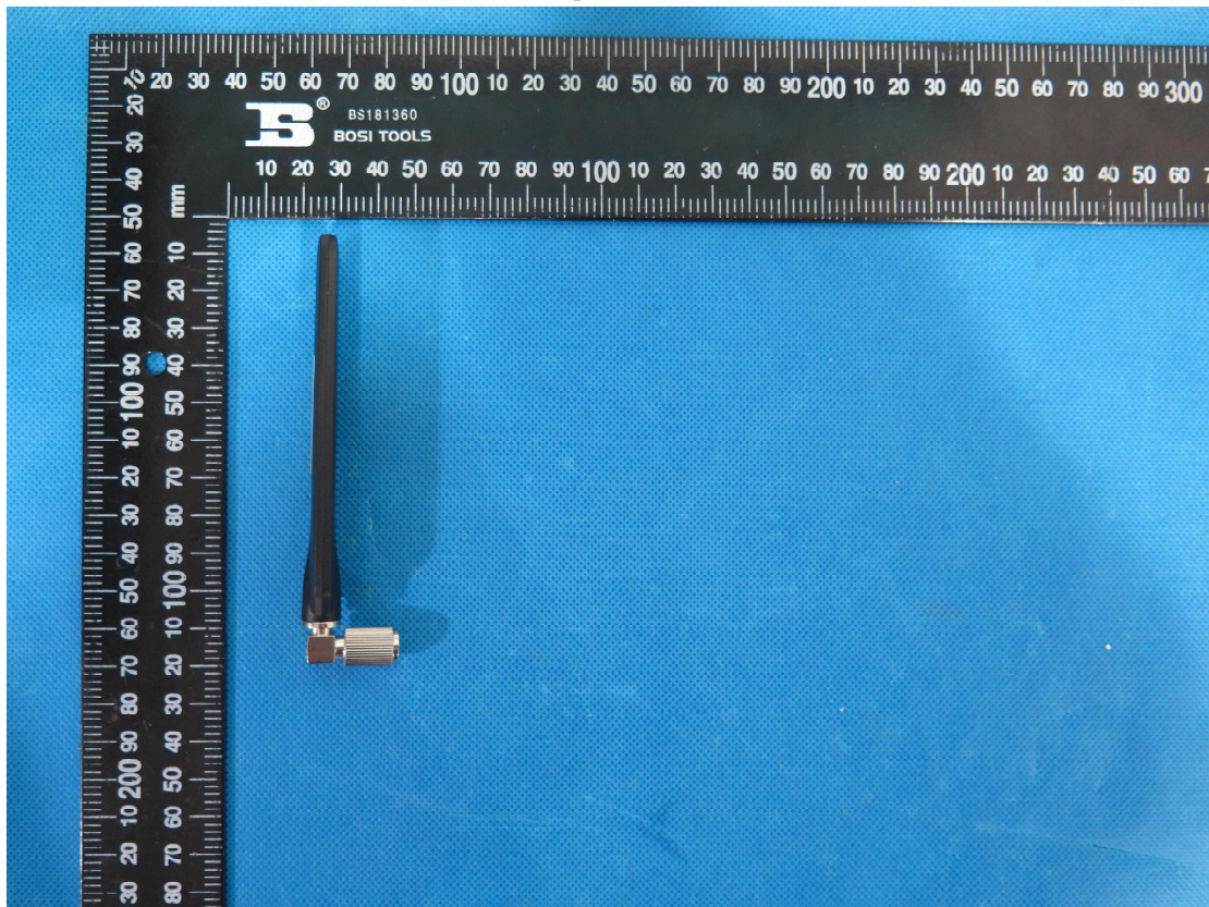
BT and LTE Antenna
