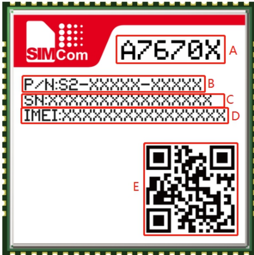
Figure 39: Label information for A7670X
