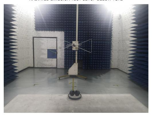
RADIATED EMISSION TEST SETUP ABOVE 1GHz
