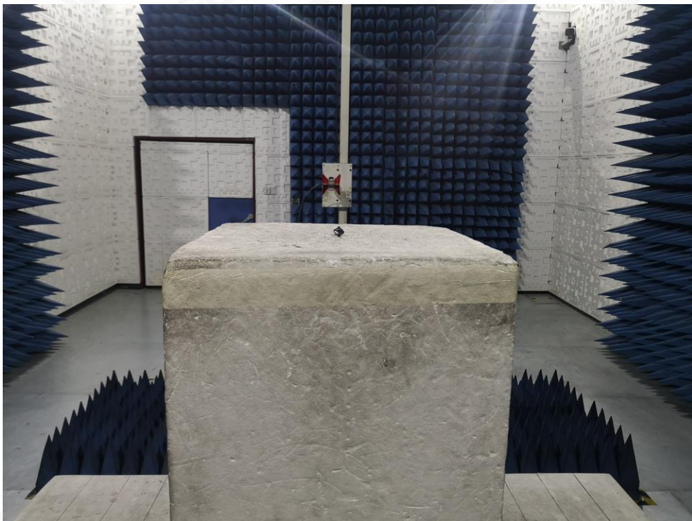
RADIATED EMISSION TEST SETUP ABOVE 1GHZ
