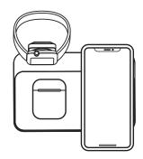
There are coils located inside the Base Station. This will allow you to place and charge your device in multiple orientations.
