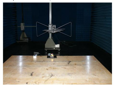
Photograph 3: Set-up for Radiated Spurious Emission, 9KHz - 30MHz
