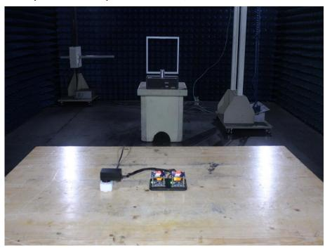
Photograph 4: Set-up for Radiated Spurious Emission, 30MHz - 1GHz
