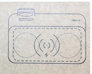
There are three charging coils located inside the Base Station. This will allow you to place and charge your device in multiple orientations.
